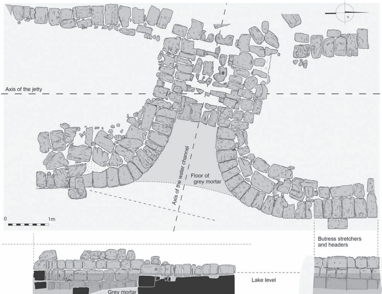
Fig. 12. Plan and elevation of the inner south face of the north flush and buttress. Lay out, drawing and DAO by M. El Amouri. © MAFT
