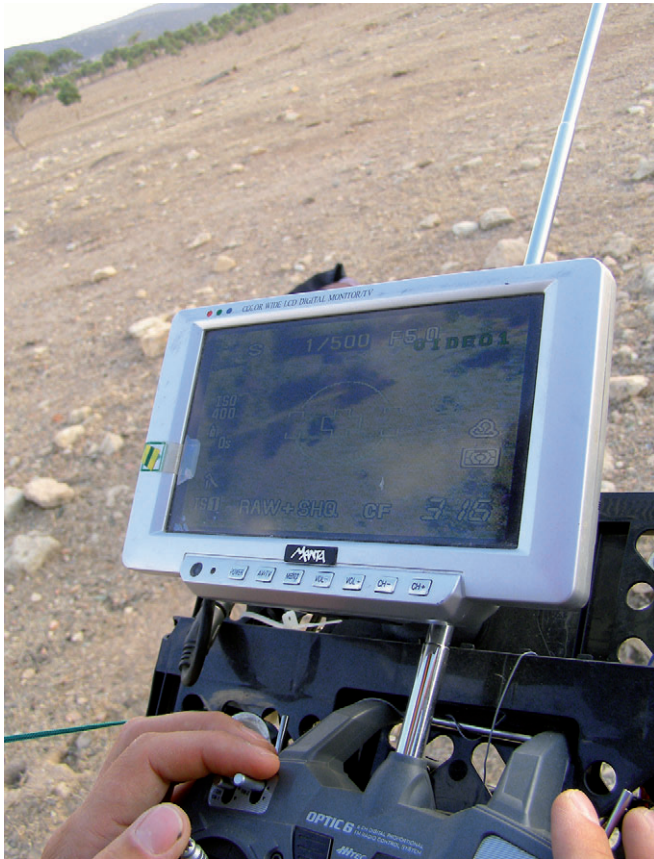
■ fig. 6 LCD panel for preview of the taken photographs
