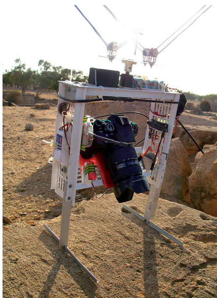
■ fig. 2 Remote-controlled camera rig
