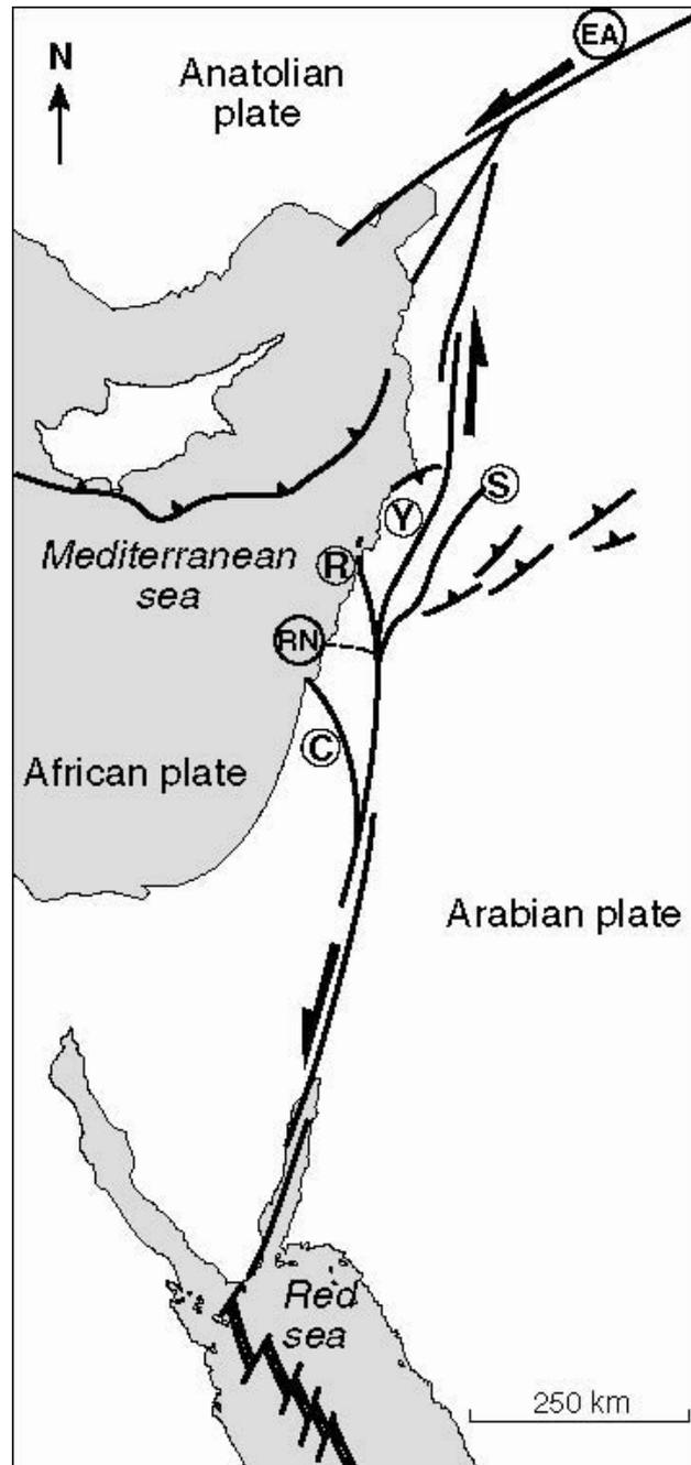
**Figure 6.10:** Tectonic setting of the Lebanese portion of the Dead Sea Transform fault system. C- Carmel fault; R - Roum fault; Y - Yammuneh fault; S - Serghaya fault; RN - Rosh Hanikra / Ras Nakoura fault, EA – East Anatolian fault.
