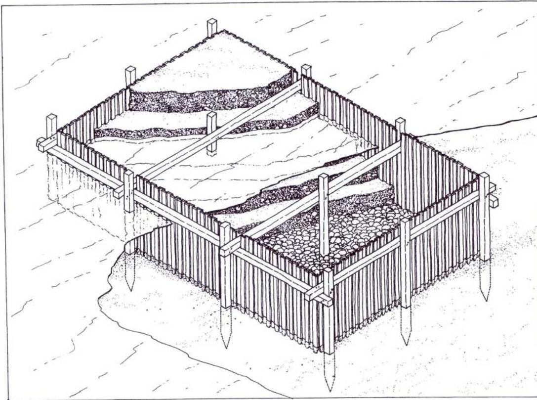
**Figure 6.7:** Roman mole Type 1. Hypothetical reconstruction after Vitruvius in Brandon (1996). This technique was widely used at Cosa and Caesarea Maritima. A slight variant is the caisson or settling barge, which was floated into position before being weighted down with ballast and hydraulic concrete.
