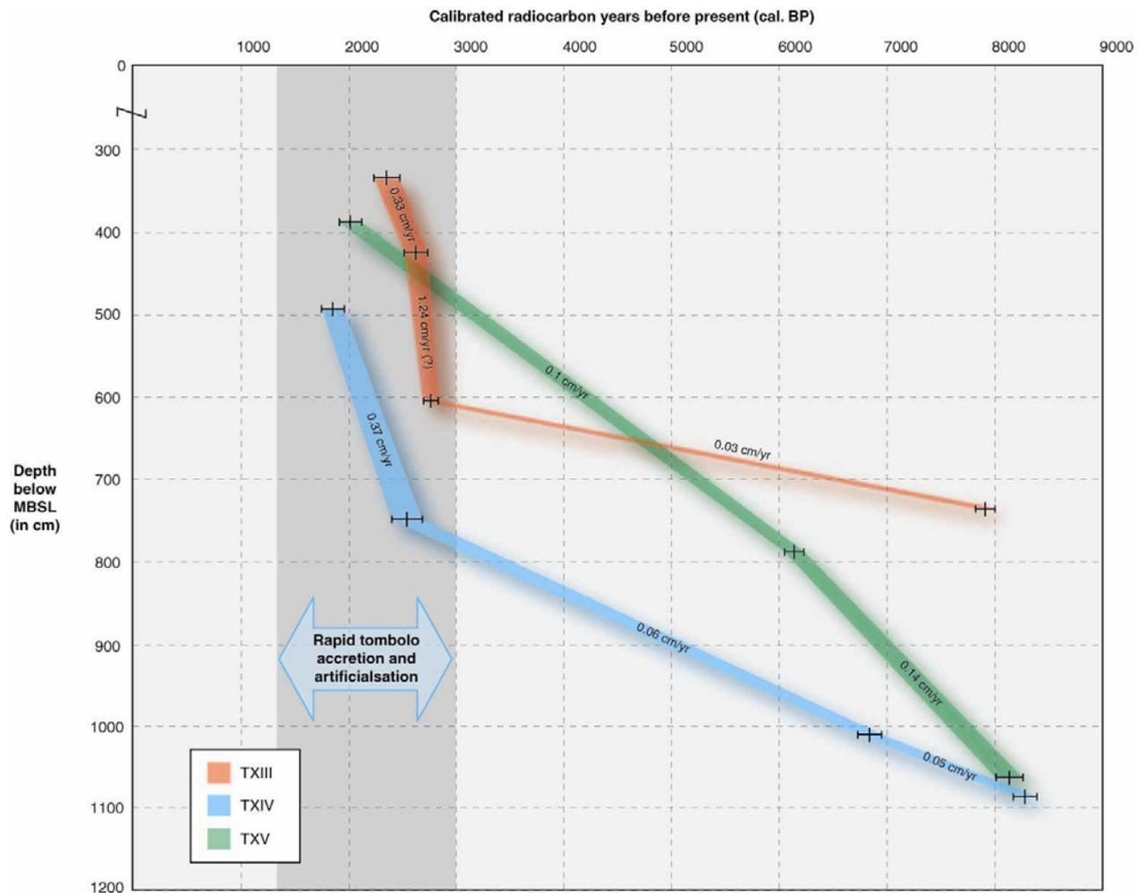
**Figure 2.45:** Tombolo accretion rates. Rapid rates of accretion,  $>0.30$  cm/yr, are attested to after 3000 cal. BP. This is attributed to anthropogenically forced erosion of surrounding watersheds, yielding increased sediment supply to coastal depocentres. This entrapment was further accentuated by an artificialisation of the salient during the Hellenistic period.
