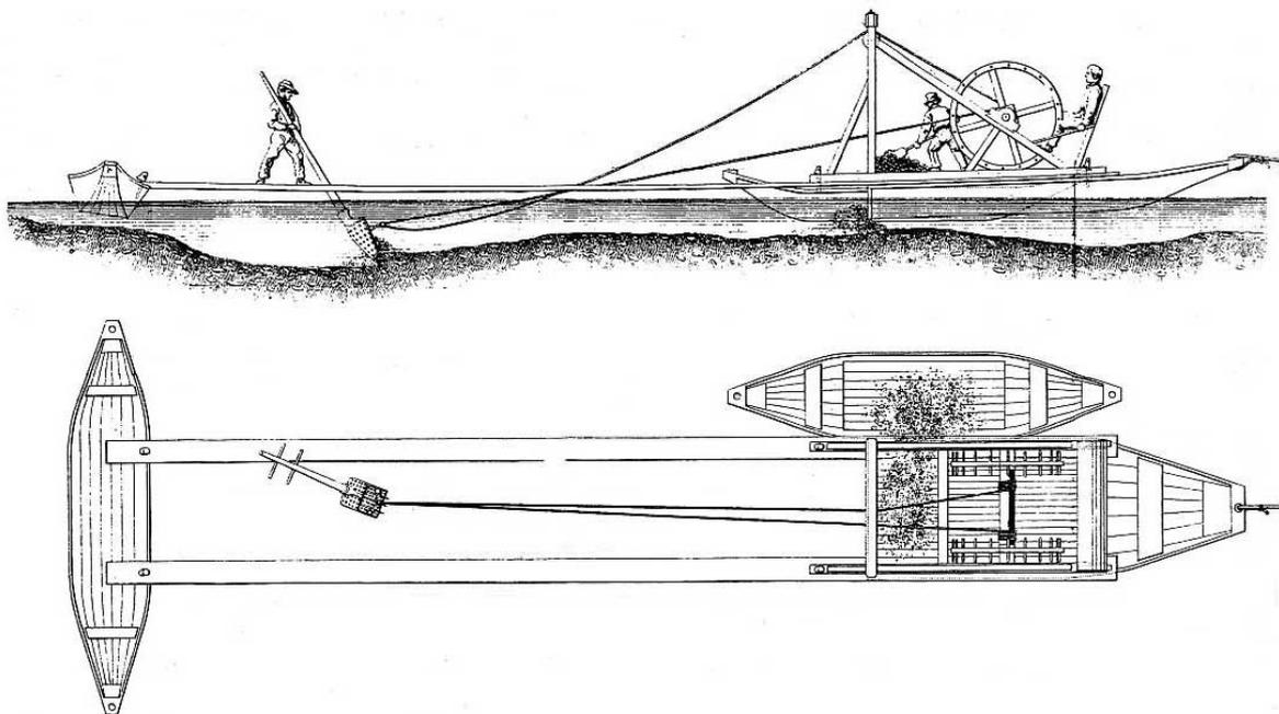
**Figure 3.31:** Eighteenth and nineteenth century dredging equipment used in European fluvial contexts. The vessel immediately adjacent to the 'pull boat' is equipped with a removable bottom, to facilitate the dumping of dredged material at a distal location. Engraving in Billaud and Marguet (2006).
