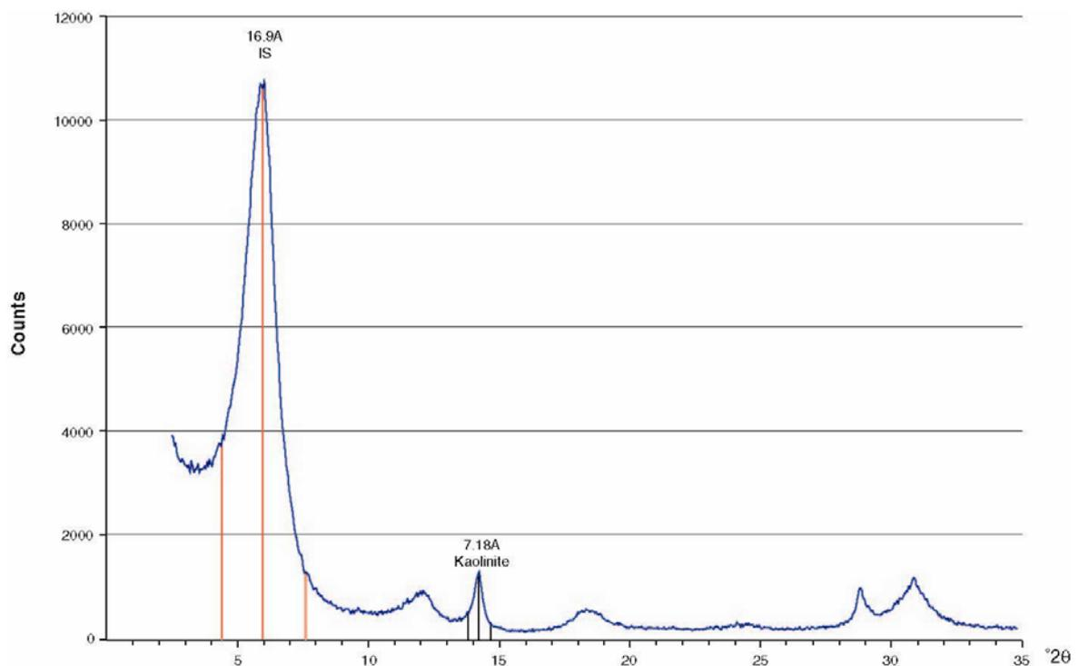
**Figure 6.37:** Diffractogram of a brown/black soil in the Tyre vicinity. The assemblage comprises dominant smectite (>80%) with low amounts of kaolinite (<20%). The deep brown/black soils are rich in expandable clays (low saddle values) that yield a very compact and prismatic structure.
