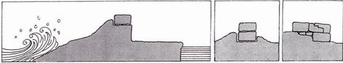
**Figure 6.5:** Schematic representation of Bronze Age/Iron Age rock cut harbour quays (in Frost, 1995). The blocks quarried on the leeward side are used to strengthen and heighten the natural reef.
