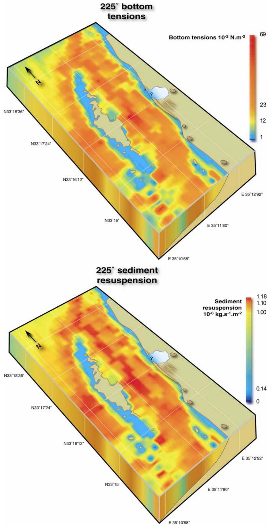
**Figure 2.12:** Model runs of wind induced bottom tensions and sediment resuspension at 5500 BP from 225°.
