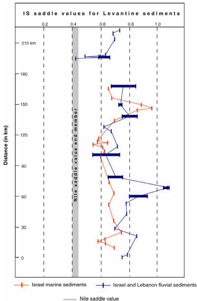
**Figure 6.33:** North-south plot of IS saddle values for fluvial and marine Levantine sediments (Israel data from Sandler and Herut, 2000). The data show a clear offset between marine and adjacent fluvial systems, especially in southern Levant. This suggests a mixing of Nilotic and local sediment sources, which remain dominant, in these areas.
