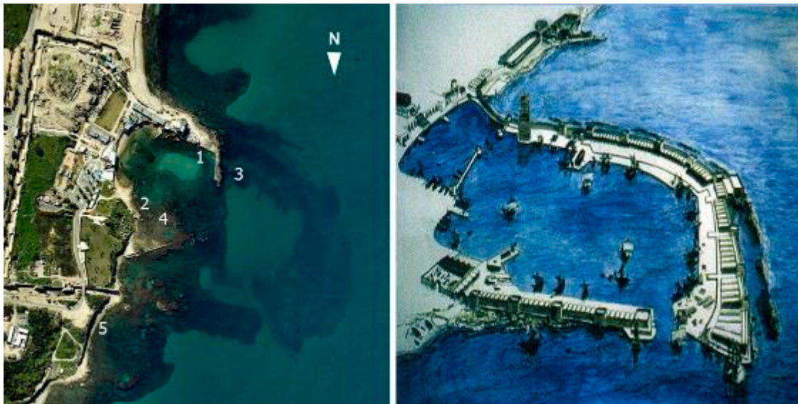
Figure 4. Left—Aerial photo of the remains of the harbor of Sebastos at Caesarea: (1) Roman dock; (2) Roman dock; (3) collapsed Roman moles, built of concrete; (4) crusader mole; (5) beach-rock deposits. Right—Artistic rendition of the harbor at the time it was built [29].
