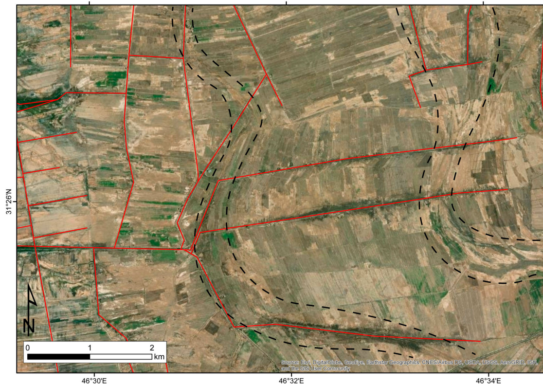
Figure 5. The irrigation canals mapped with red lines partially overlap the inactive fluvial channels traced by black dotted lines.
