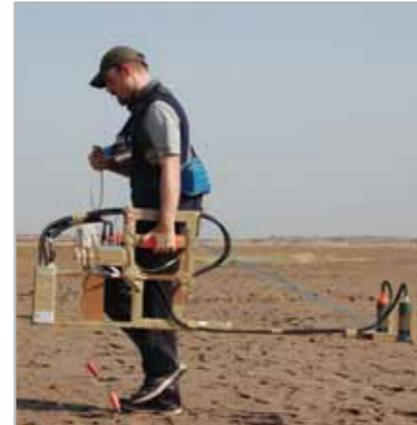
Martin Gruber surveying at Charax. The caesium magnetometer is designed to be easily dismantled and transported.
