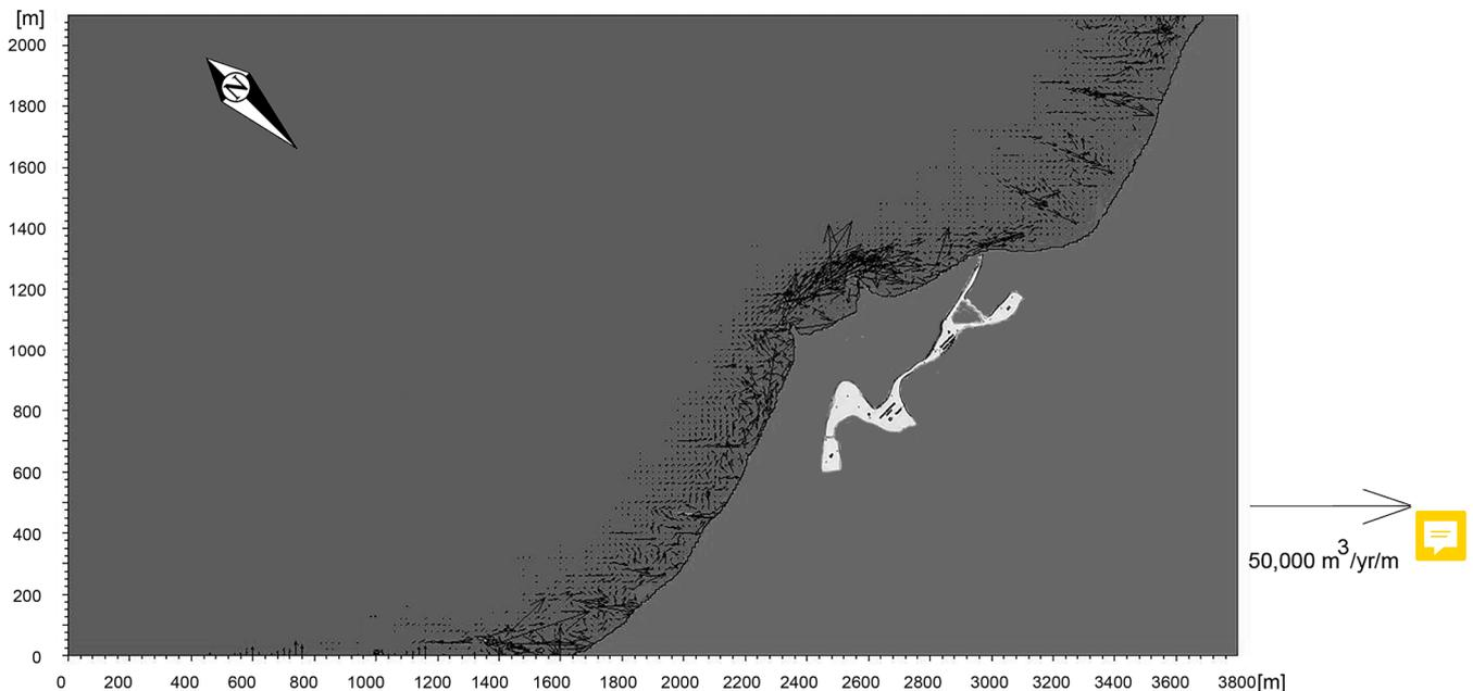
Figure 11. Simulation of sediment transportation, for north-westerly wind. Area of the inland basin and the entering channel are also shown.
