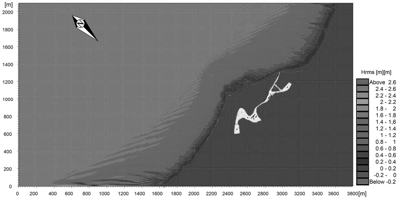
Figure 9. Simulation of wave field (PMS) for north-westerly wind. Area of the inland basin and the entering channel are also shown.
