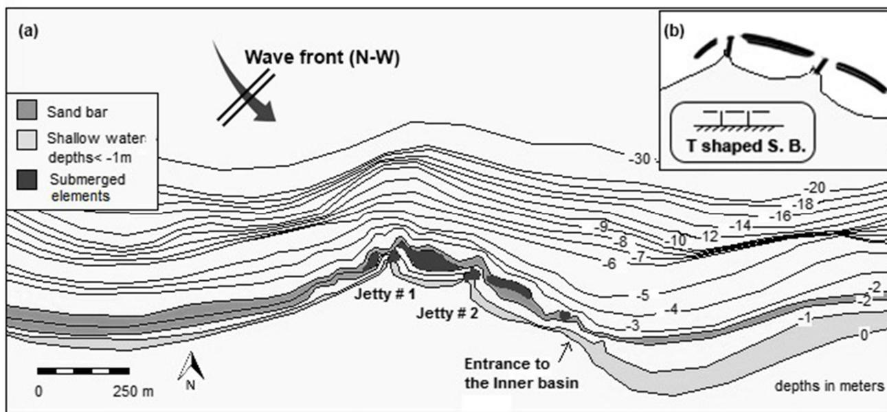
Figure 5. (a) Bathymetry and location of the submerged structures and natural reefs, functioning as sediment transport controllers. (b) Configuration of the T-like shaped plan of the submerged breakwaters system. Image plotted by adjusting two bathymetry maps, i) from the Hellenic Navy Hydrographic Service (scale 1:100,000), ii) (scale 1:10,000), by a study of Papafiotiou (2008).
