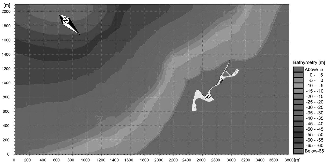
Figure 8. Bathymetry model turned by 45° anti-clockwise. Area of the inland basin and the entering channel are also shown.
