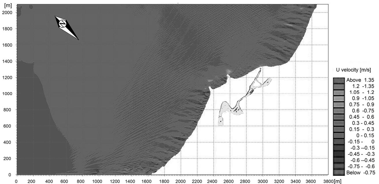
Figure 10. Simulation of horizontal hydrodynamic velocities (U), for north-westerly wind. Area of the inland basin and the entering channel are also shown.
