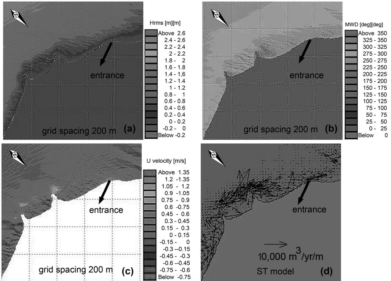
Figure 12. (a) Wave heights, (b) Mean wave direction change, (c) Horizontal velocities field, (d) Sediment transportation flow, for north-westerly wind.
