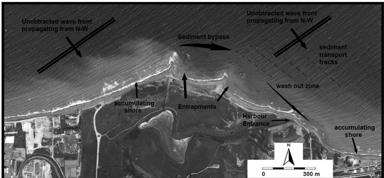
Figure 7. Sediment transportation mechanism during a wind storm event (2012, Google earth imagery).
