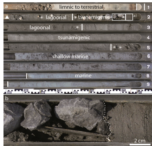
Fig. 2: (a) Vibracore LEC 2 ( N 37^{\circ} 55' 58.6 E 22^{\circ} 53' 03.5'' , -0.04 m a.s.l.) was drilled in the central Lechaion harbour basin. Here, two coarse-grained tsunami layers were found, intersecting the autochthonous, predominantly shallow-marine to lagoonal facies. Youngest tsunami deposit as encountered in core LEC 3 and covering early Christian basilica is dredged at site LEC 2 (see \Delta ). ^{14}C -samples are marked by *. (b) Detailed view of the younger event layer. The quiescent harbour environment was abruptly covered by allochthonous high-energy deposits (Photo by T. Willershäuser, 2010).
