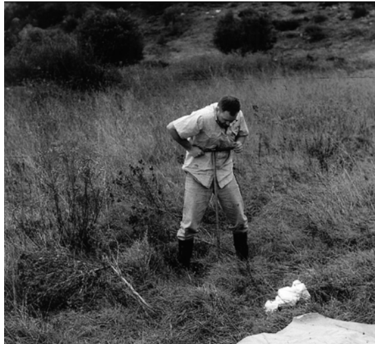
Figure 7. Dr Rick Dunn conducting his geological survey of Torone's floodplain by way of hand-augering.
