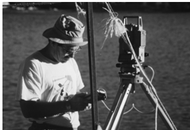
Figure 4. Dr Tony Sprent at the 'Total Station', an electronic theodolite allowing a three-dimensional survey of 'Area 1'
