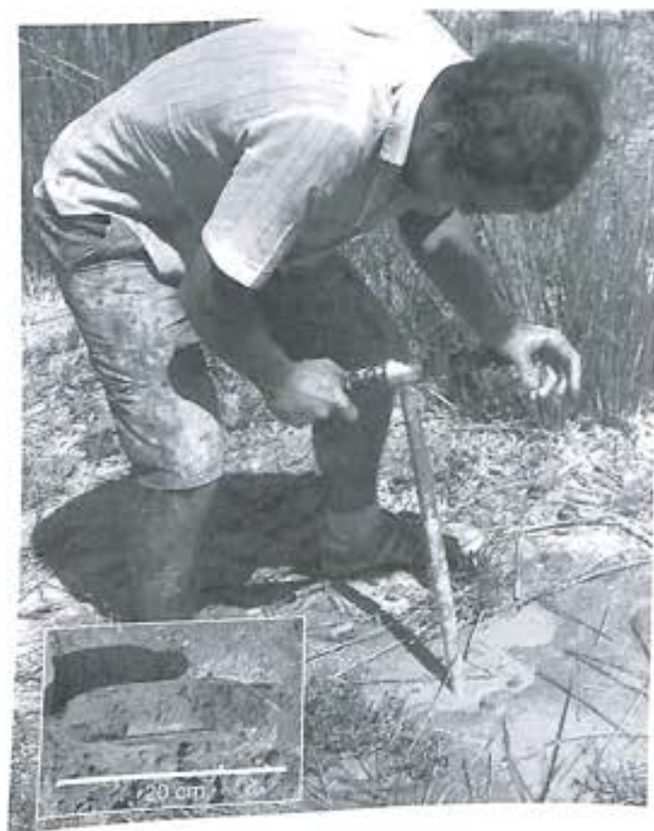
Fig. 5.7. Photograph of auger in use and resulting core sample (in insert). Penetration is allowed by both turning and pushing the auger into the soil. Even if it obliterated sedimentary structures, stratigraphy is well preserved. The flexibility and ease of use of the Edelman auger allows multiple points to be studied in the same day (LMRP/C. Flaux).
