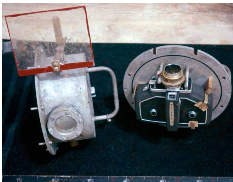
Figure 1.6. The underwater movie camera case, made in the engineering laboratory at Cambridge, disassembled to show the internal arrangement. The external view-finder is designed to match the wide-angle lens that is shown in the picture. The scale bar is in cm.
