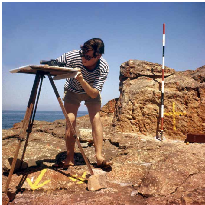
Figure 1.8. Nick Wood working with the telescopic alidade on the tripod, positioned on the West Island. The yellow arrows permit the tripod to be put in exactly the same place on different days. Nick is viewing a diver in the sea holding a coloured ranging pole, like the one in the background.
