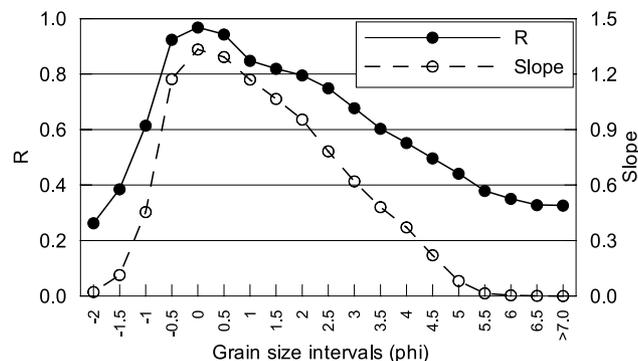
Fig. 6. Relationships between carbonate contents and grain size. Y-axis (right): slopes of relations between cumulative grain size classes and carbonate contents. Y-axis (left): associated correlation coefficients.
