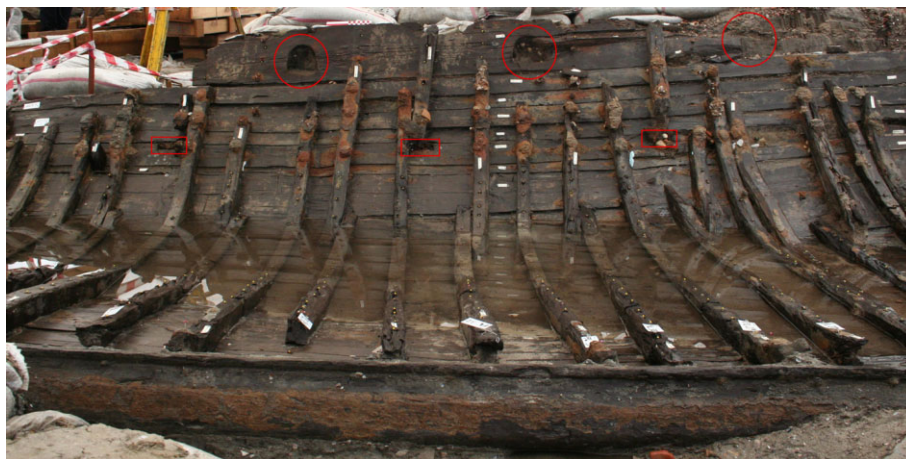
Figure 33. Port side of galley YK 4, view from interior; oar-ports are circled, and bench notches are highlighted with rectangles; November 2006. (Photo M. Jones/INA)
