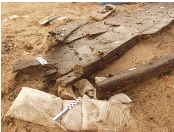
Figure 22. In situ repair timber on the keel of YK 24 (YK 24 Keel 1); July 2007. (Photo M. Jones/INA)
