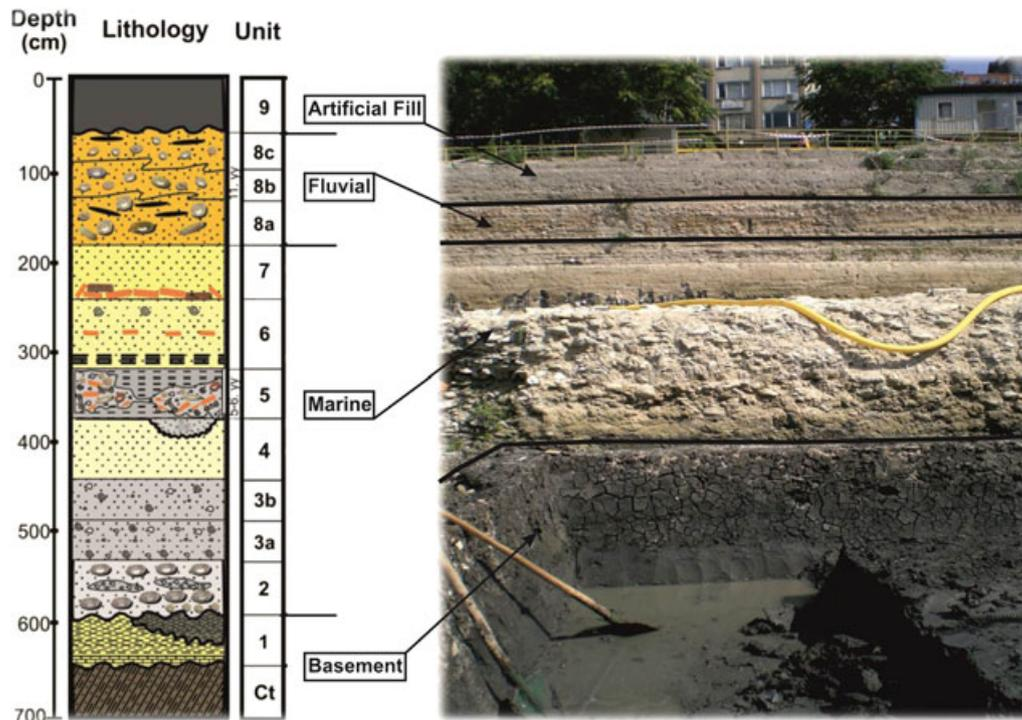
**FIGURE 4** Generalized stratigraphic section and view of the sedimentary sequence uncovered in Yenikapı-Istanbul by salvage excavations. (Ct) is the Trakya Formation of Carboniferous age, encountered in deeper bore-holes drilled for engineering geological purposes [Color figure can be viewed at [wileyonlinelibrary.com](http://wileyonlinelibrary.com)]
