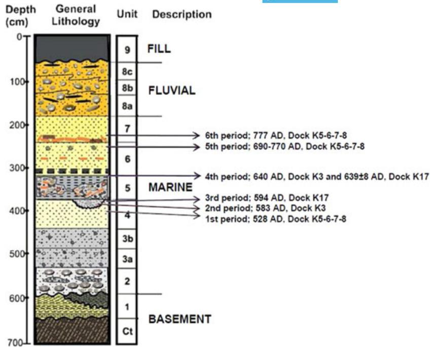
**FIGURE 8** Position of equivalent stratigraphic intervals of six periods according to the results of dendrochronology. The positions of periods 4 and 6 are not indicated by a disconformity because the respective units had already been excavated before this study [Color figure can be viewed at [wileyonlinelibrary.com](http://wileyonlinelibrary.com)]
