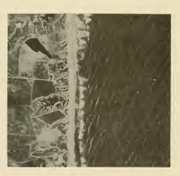
simultaneously forming an irregular pattern of short-crested waves. The right photo shows long swell obscured by local wind waves until almost the breaking point.) Waves in a coastal region. (The left photo shows two wave trains approaching the shore Figure 3-2.
