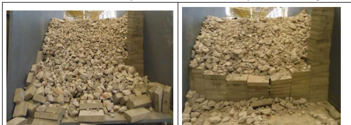
Figure 7.4 Example dry-build failure
