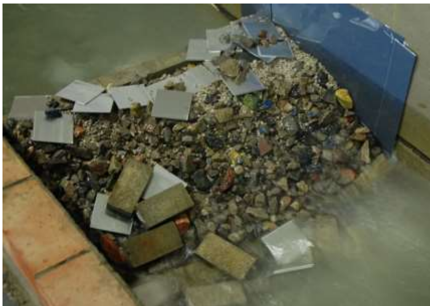
Figure 7.29 Section 5 after collapse of the seaward wall
