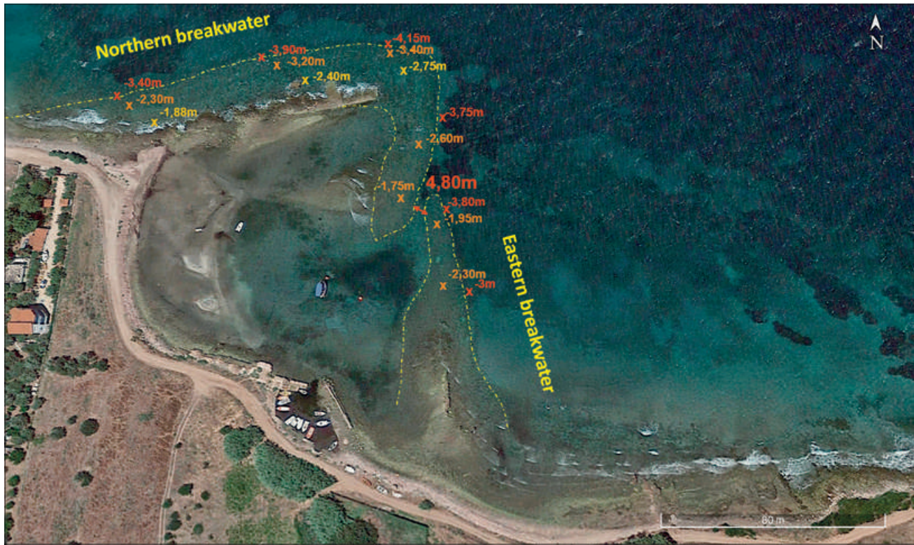
Fig. 8 Measurements of the breakwaters and of the entrance of the harbour of Anthedon. – (Photo A. Ginalis, 2018).
