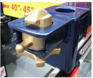
Twist-lock on a rear corner of a container semi-trailer; the container corner is placed over it and it has to be turned 90° to close the lock (picture Wikipedia).
