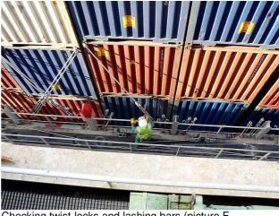
Checking twist-locks and lashing bars (picture F. Massard, 2007).
