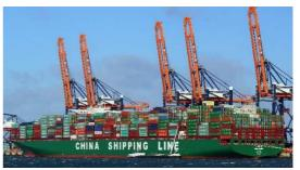
Five gantry cranes with arms lifted allowing ship movement. A berth of this type can move around 150 TEU per hour (picture <a href="https://www.marinetraffic.com">https://www.marinetraffic.com</a>).
