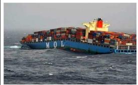
MOL Comfort (316 m long) broken in two parts during a storm in the Indian Ocean and sunk in June 2013 (picture <a href="http://www.meretmarine.com">http://www.meretmarine.com</a>).
