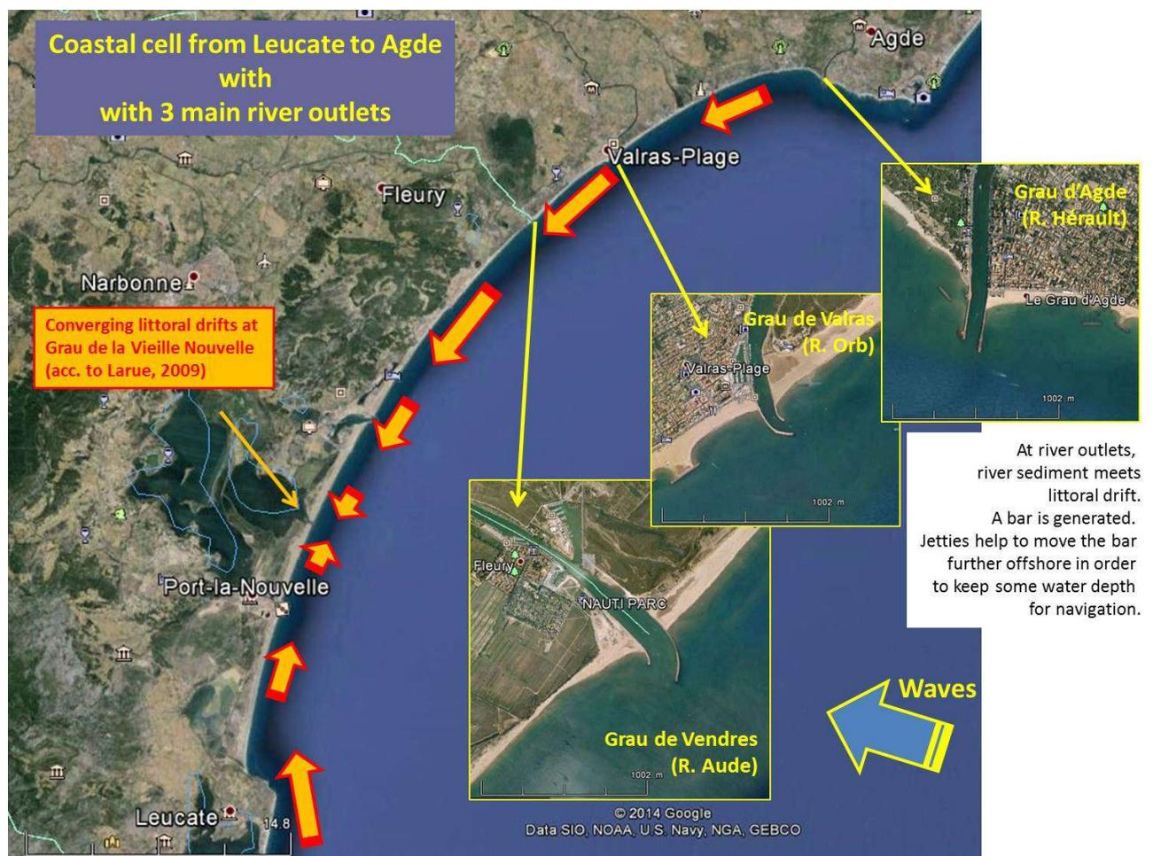
Littoral drift is due to oblique wave incidence on the coastline (Larue, 2009, Kulling, 2017).
