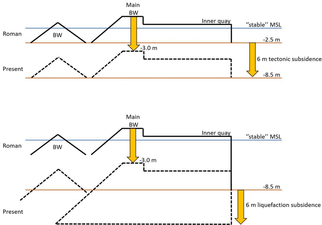
Schematic options for subsidence of the Caesarea main breakwater.
