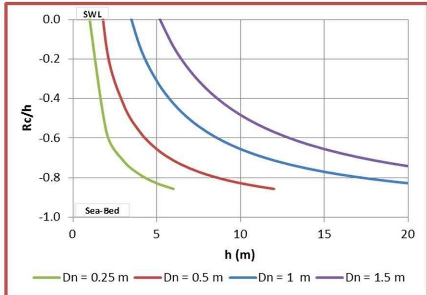
Stable submerged breakwater with breaking waves
