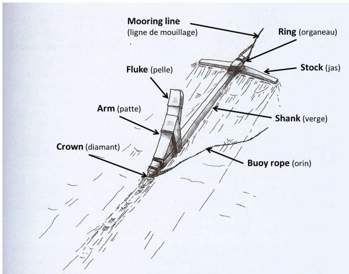
Functioning of a wooden anchor with lead stock
