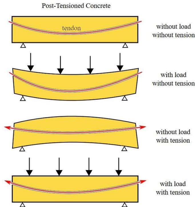
The vertical load induces tension in the lower layer of the beam.
