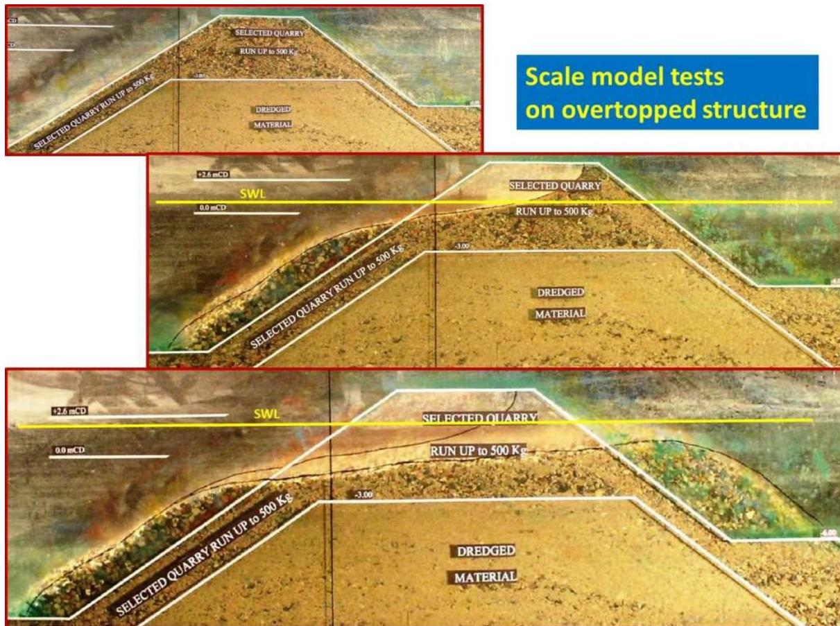
Reshaping of an overtopped rubble mound breakwater by wave action
