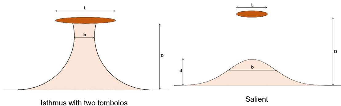
L is the length of the island and D is the distance from the initial shoreline. For isthmuses, we define b as the smallest width of the isthmus, and for salients, b is the width at the inflexion point, and d is the distance from the tip of the salient to the initial shoreline.
