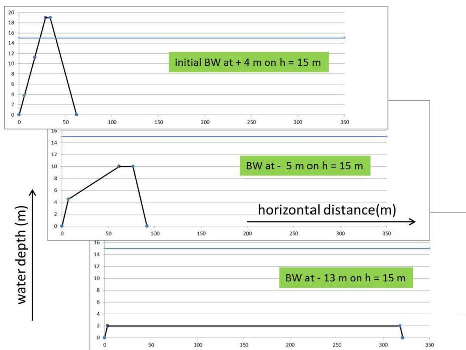
Destruction of a breakwater due to wave action.
