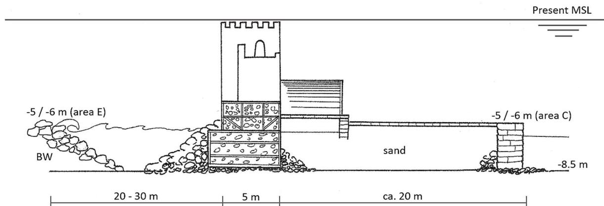
Cross-section of the main breakwater (adapted from Raban, 2009:96).
