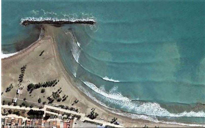
Wave diffraction pattern behind a detached breakwater
