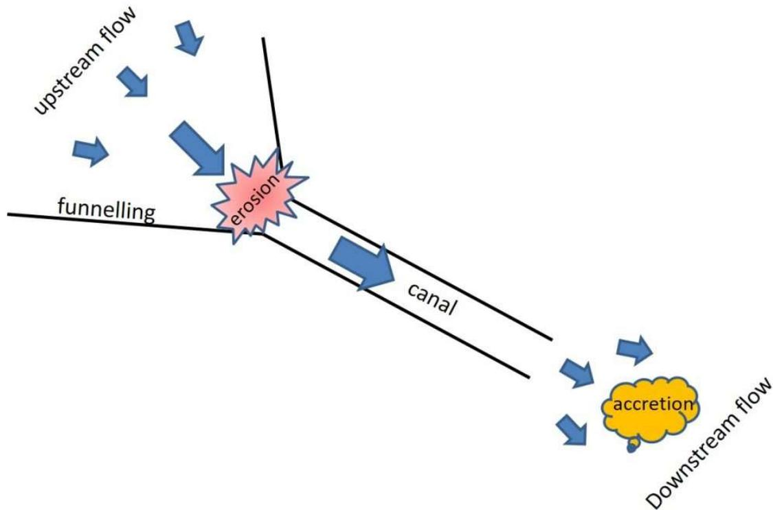
Sediment transport in a canal showing erosion at the intake upstream, and accretion at the outlet downstream.
