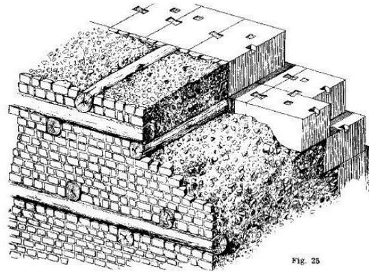
Concrete reinforced with timber,
