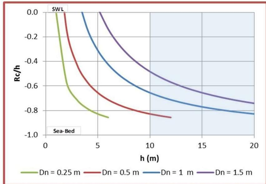
Stability of stones according to water depth and rubble mound crest level
