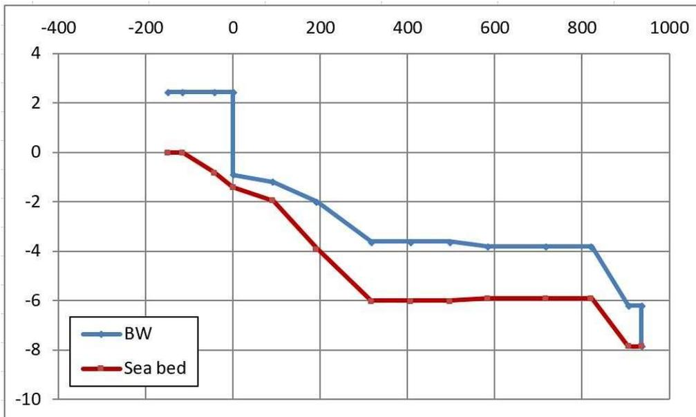
Longitudinal profile of the main breakwater (BW)
