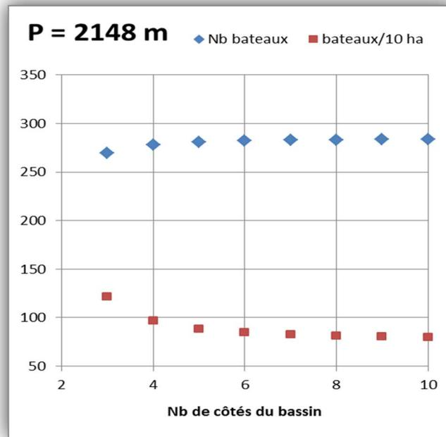
Computation of the number of ships in a polygonal basin with n sides.
