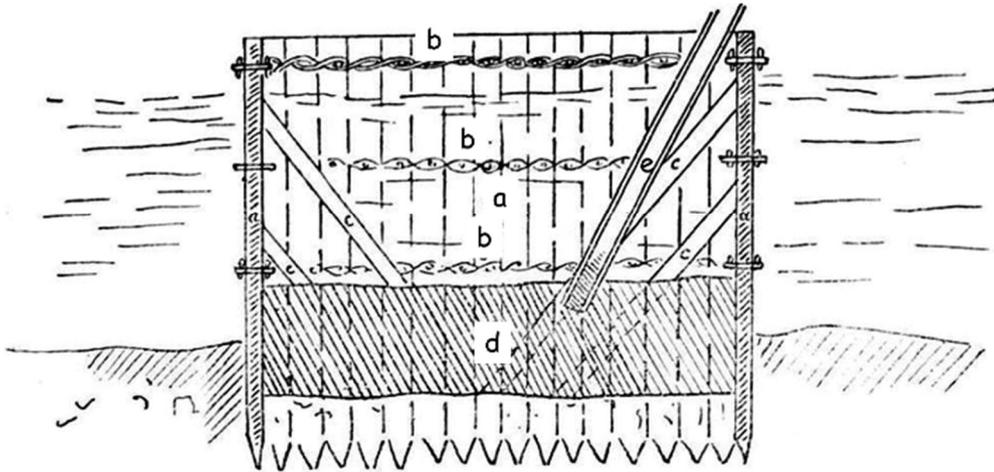
Ch. Dubois' sketch, "Observations sur un passage de Vitruve, Mélanges d'archéologie et d'histoire T. 22" (1902) with a system with adjacent poles (a) connected (or even engirdled) by chains (b). However, his system with chains and oblique tie rods does not seem realistic: the rods must be horizontal and connecting opposite caisson faces like Brandon suggested in 1996.
