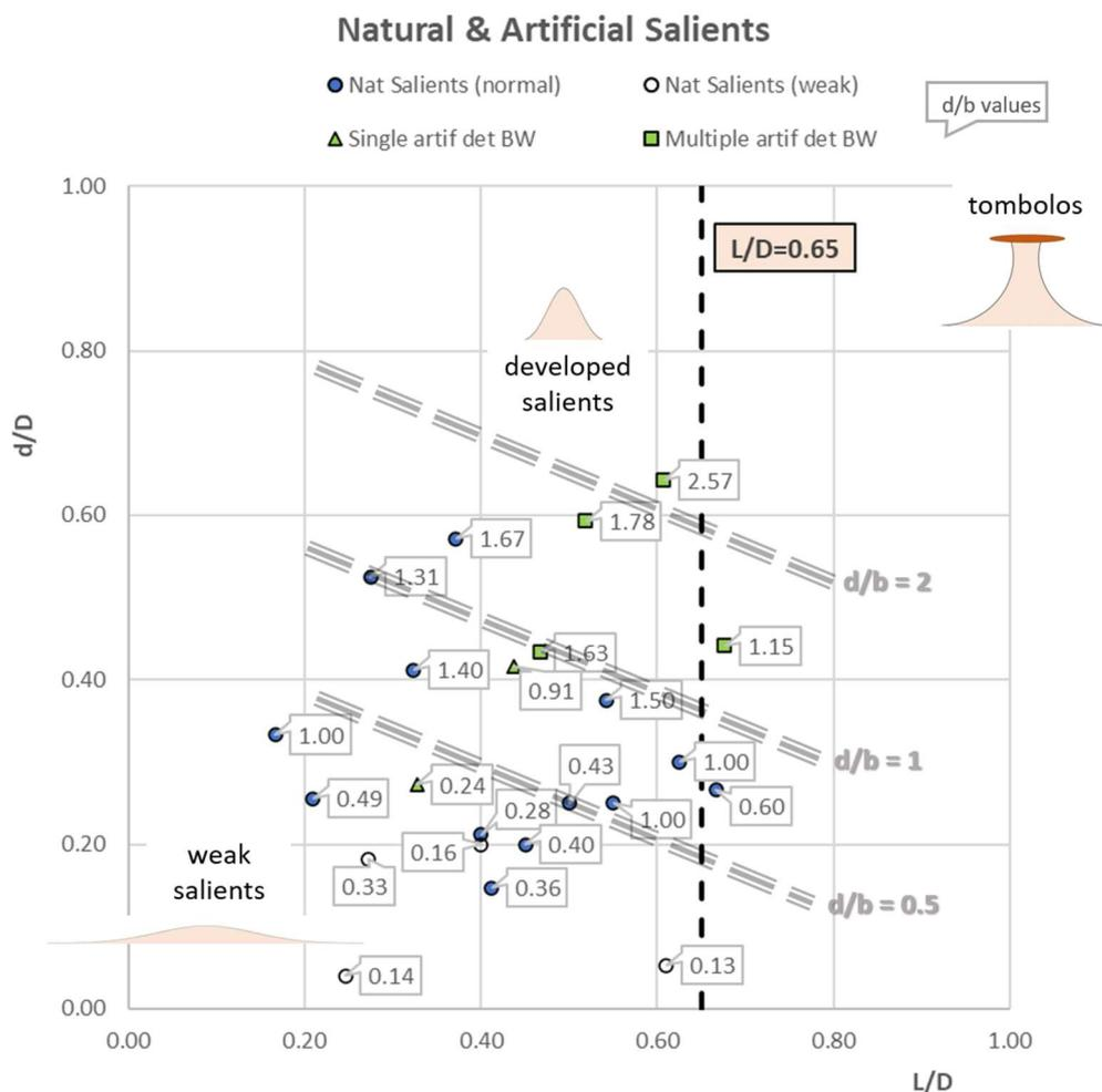
$L/D$  for salients, including both natural and artificial man-made structures (for  $L/D < 0.65$ )
