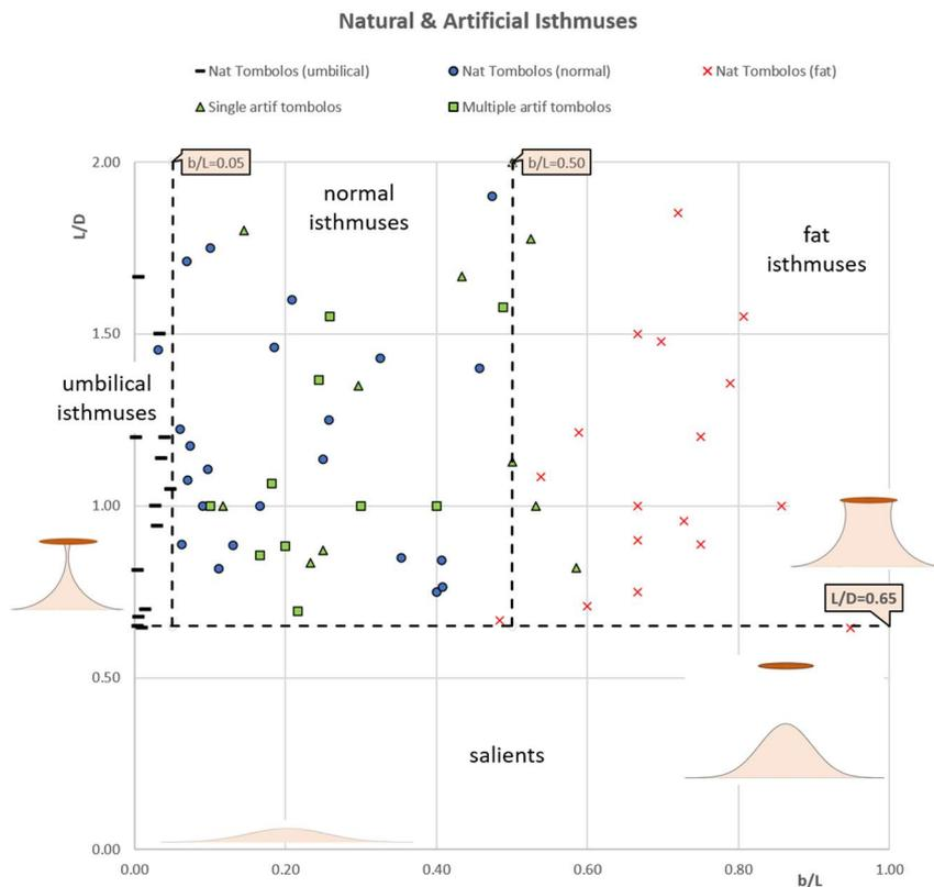
$L/D$  for isthmuses with tomboles and for salients, including both natural and artificial man-made structures (for  $L/D < 2$ )
