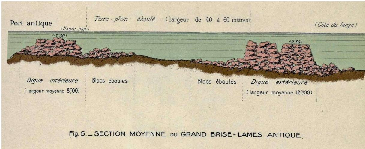
Fig. 2: Jondet's cross-section of the main north breakwater.
