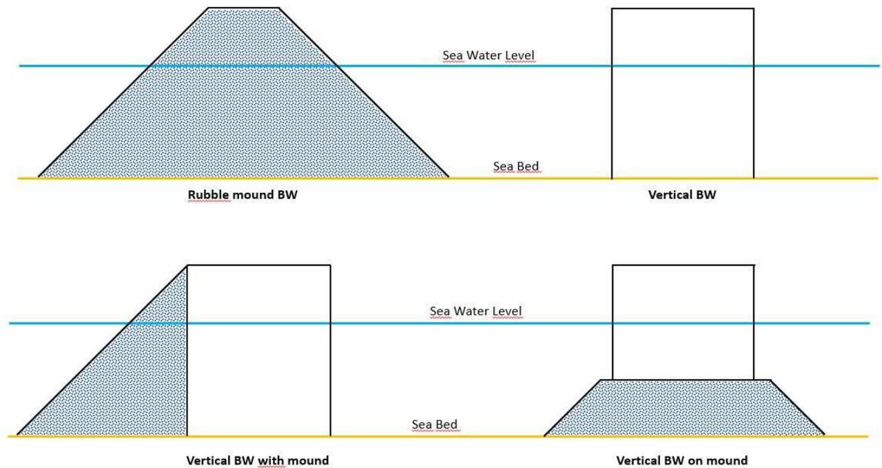
Cross-section of various types of breakwater
