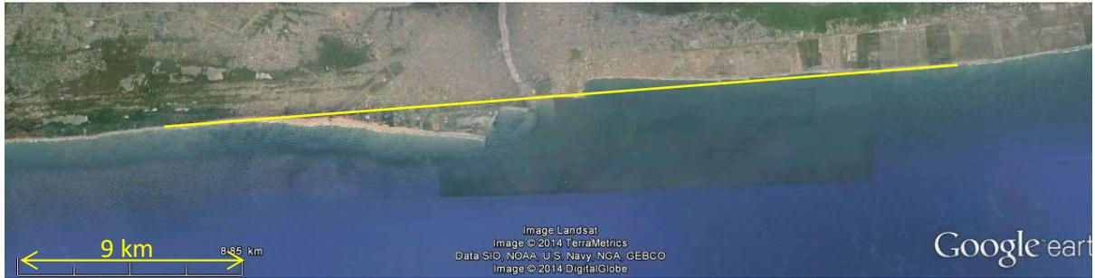
This picture shows the initial shoreline near Cotonou (Benin) (straight yellow line). This was the shoreline before any human construction (a port) was built in the sixties. This coast is known for its littoral drift of around one million cubic meters per year from west to east (left to right on the picture).
