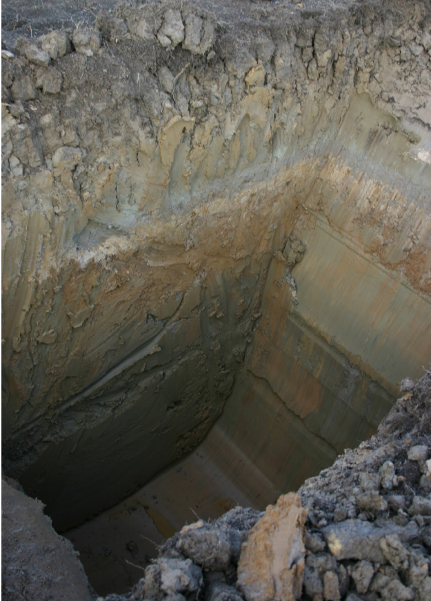
Fig 3.10 Photograph of gravels of Group II beneath finer-grained Group III sediments in GTP15
