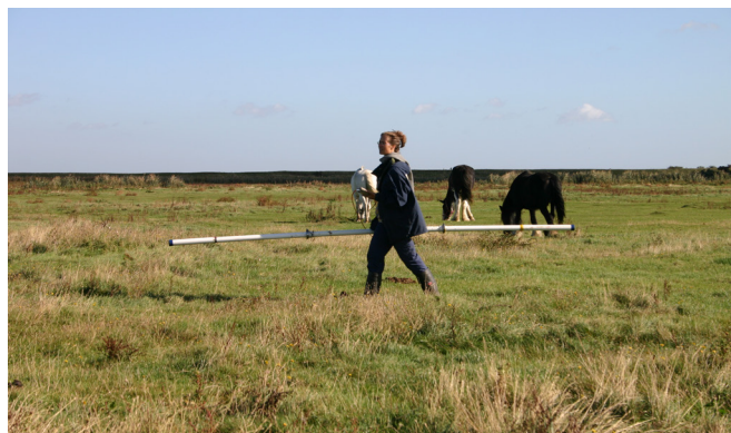
Fig 3.5 Photograph of EM 31 geophysical survey in progress
