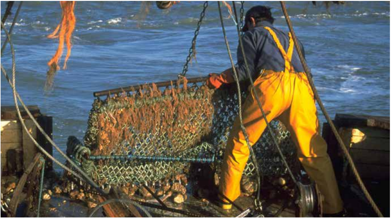
Figure 86 Recovery of an oyster dredge. Note the 'teeth' that comb the top c. 100mm of the seabed to 'tease' out the oysters
