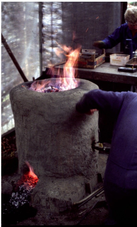
ILLUS. 4 Experimental iron smelting by Peter and Susan Crew at Plas Tan Y Bwlch, Snowdonia National Park, using bog ore from the Foulness Valley (Photo: P. Halkon)
