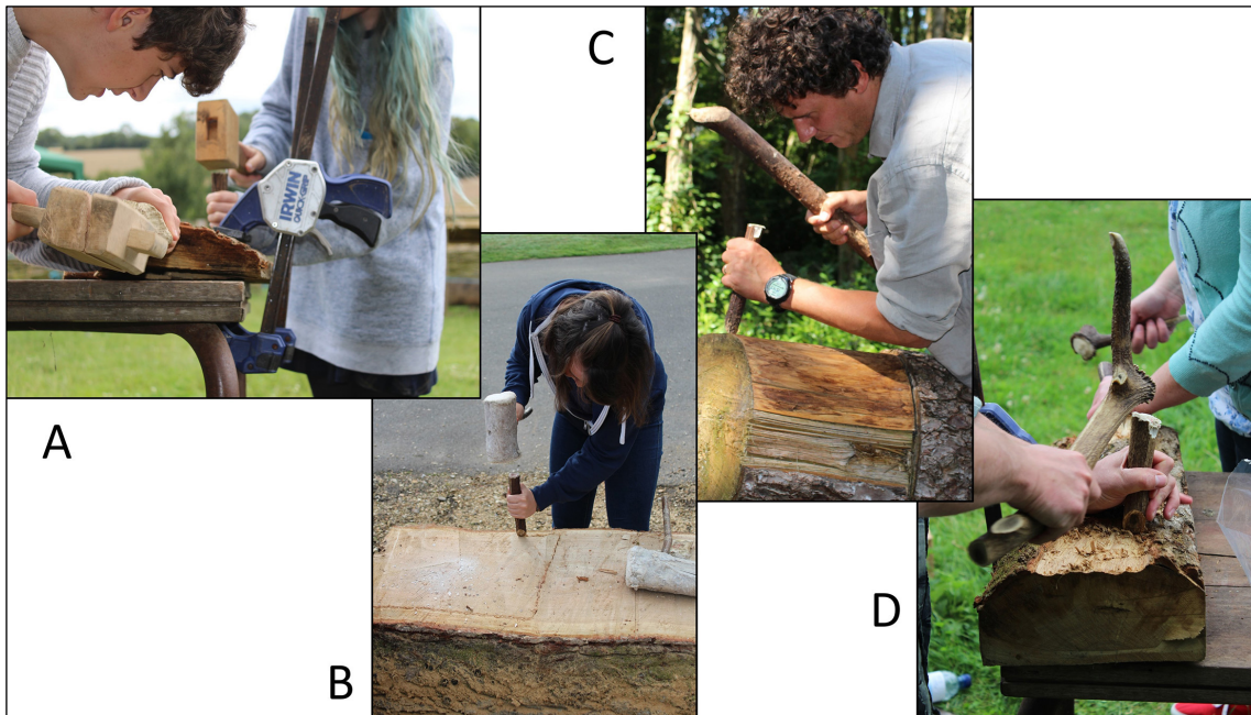
Figure 7. Experimental tangential splitting of an oak log.
