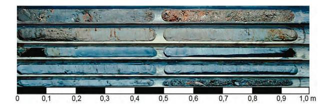
**Fig. 21.** Coring Mil 145, directly on the geomagnetic anomaly running south from the eastern harbour lion (see Fig. 17, anomaly B). The surface of the silted up harbour is in the upper left corner. Total coring depth: 5 m, diameter of open auger heads: 6 cm  $\emptyset$  (0-2 m), 5 cm  $\emptyset$  (2-4 m), 3.6 cm  $\emptyset$  (4-5 m). Note the red brick layer at 0.45-0.63 m below surface. Photograph: H. Brückner (September 2001)
