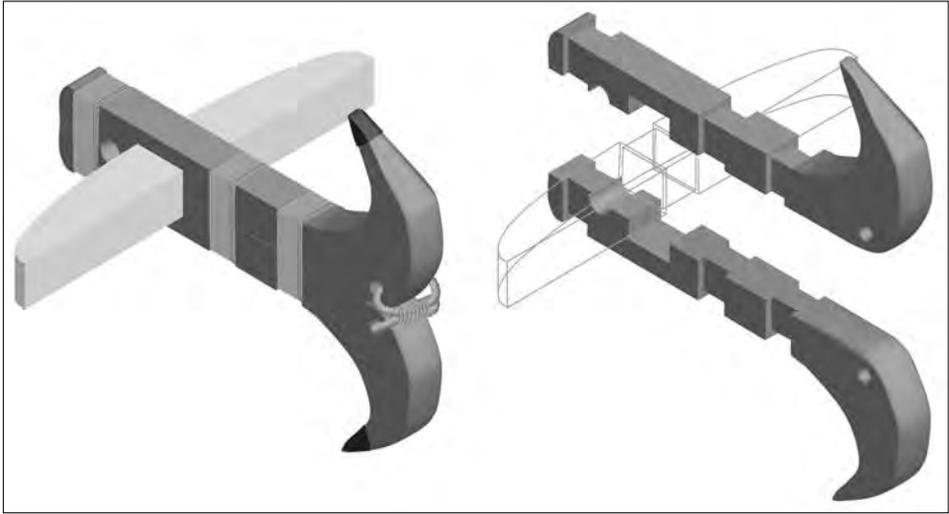
FIG. 9. Hypothetical illustration of the architecture of a stone-stocked wooden anchor. (G. Votruba).
