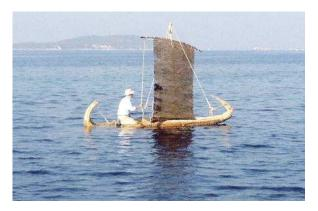
Fig. 6: Reed boat prototype. (Photo: Mualla Erkurt, November 2013, Urla). Length: 4.50m Beam: 1.10m Draft: 20 cm Sail surface: 4.5 m2
