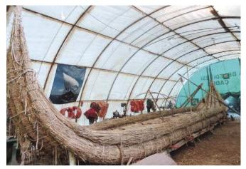
Fig. 7: Large reed boat. (Photo: Mualla Erkurt, November 2013, Urla). Length: 14.5m Beam: 2.60m Draft: 35cm Sail surface: 40 m2
