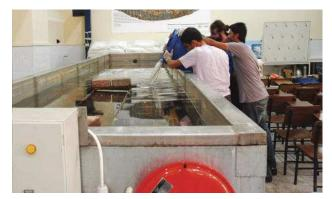
Fig. 17. PEG solution is being poured into the conservation tank.
