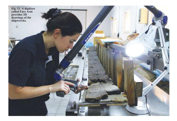
Detailed recording of the surviving ship timbers are made with a 3-D digitizer called, *FaroArm* are made. This technology has been used in the field of archaeology for the first time in Turkey by Istanbul Universityís Project team (**Fig. 11**). Ascertainable details of each timber, such as fastenings, joints, angles, tool marks, corrosion stains, etc. are all recorded using the laser scanner. Each digitized timber can then be used to create 3-D images of ship timbers<sup>10</sup>.
