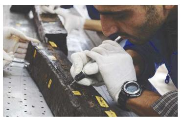
Fig. 15. Chemical and mechanical cleaning on keel before conservation.
