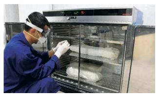
Fig. 16. Woods are being conservated by using Kauramin method.
