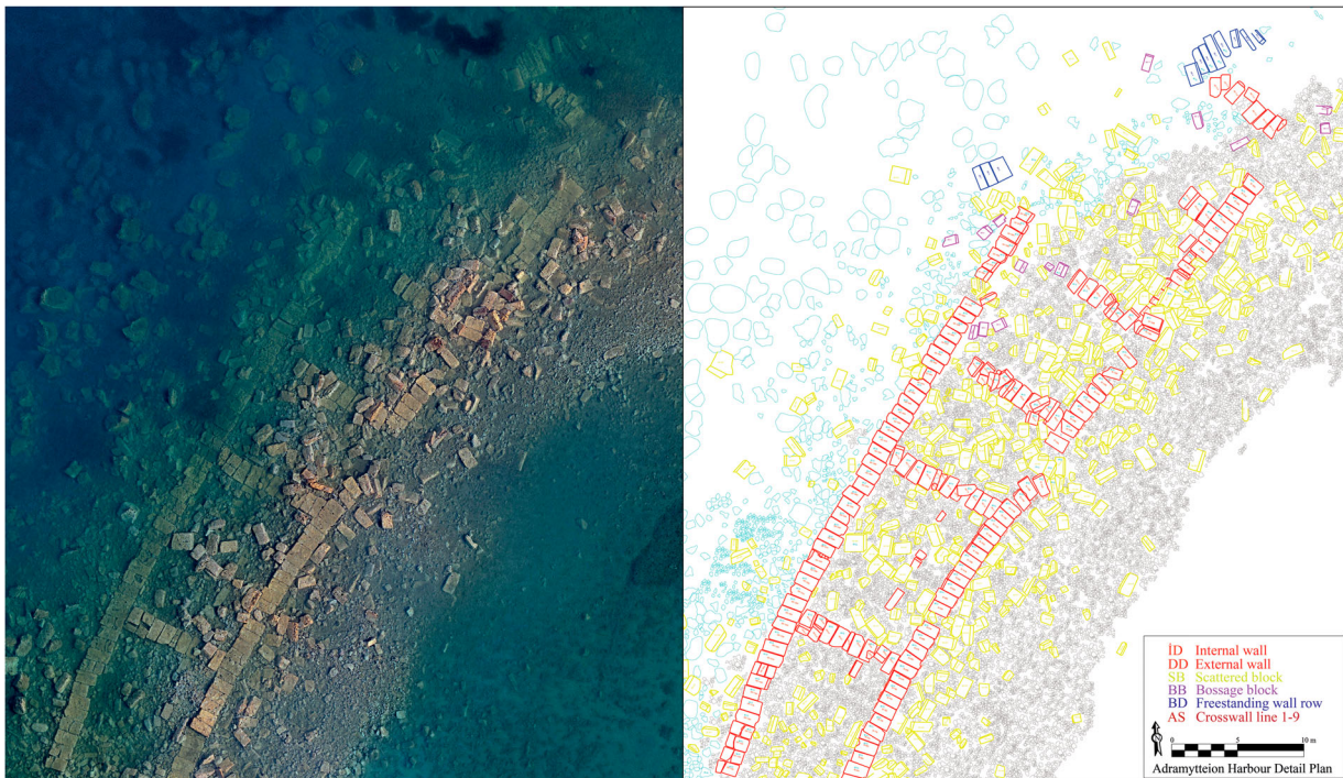
Figure 4. Detail of the crosswalls.
