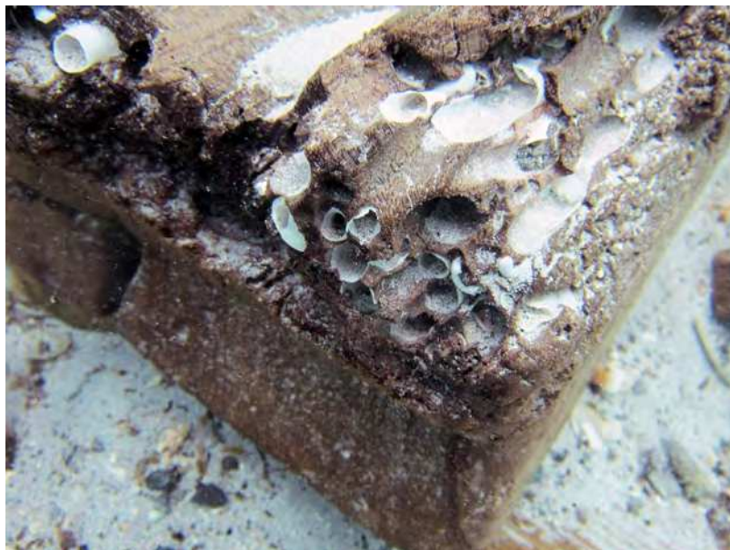
Figure 3. Detail of the end of a frame affected by the Teredo Navalis .
