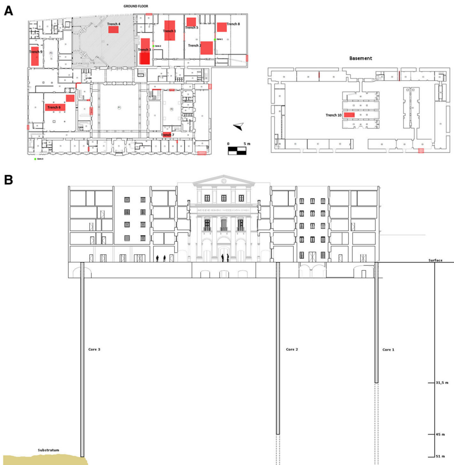
Fig. 4 Location map of the ten archaeological trenches and the three geoarchaeological corings carried out in the Valcárcel Building (a), and section view of the Valcárcel Building façade with the three corings and the location depth of the bedrock—Core 3 (b)
