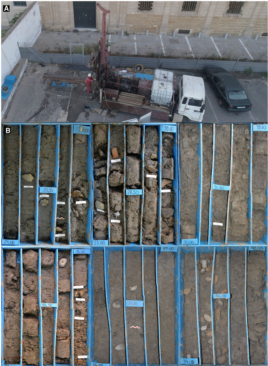
Fig. 5 Photographs showing the execution process of the geoarchaeological drillings—Core 3 (a); with a detail of the archaeological findings in Core 2 at depths between 24 and 42 m below the surface (b)
