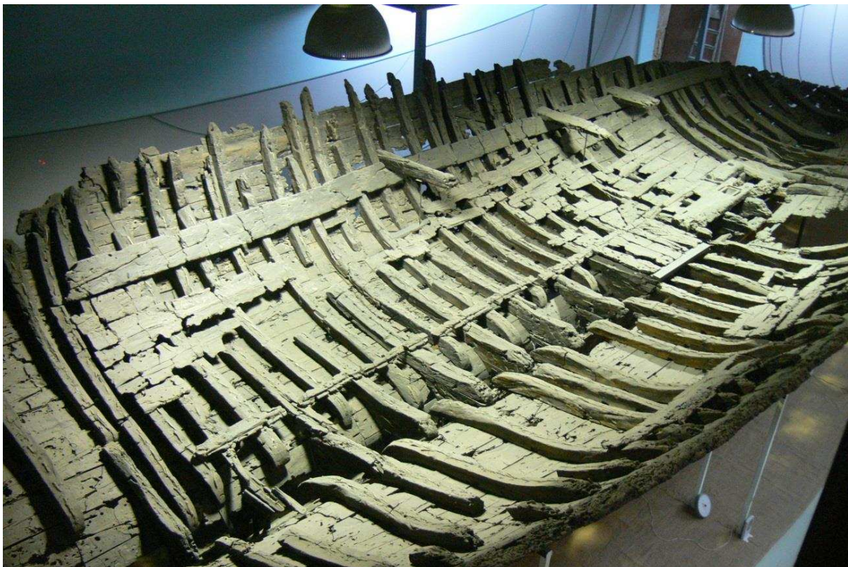
FIGURE 7. Kyrenia Ship showing common construction features of a mortise-and-tenon hull (Courtesy of Robin C.M. Piercy)
