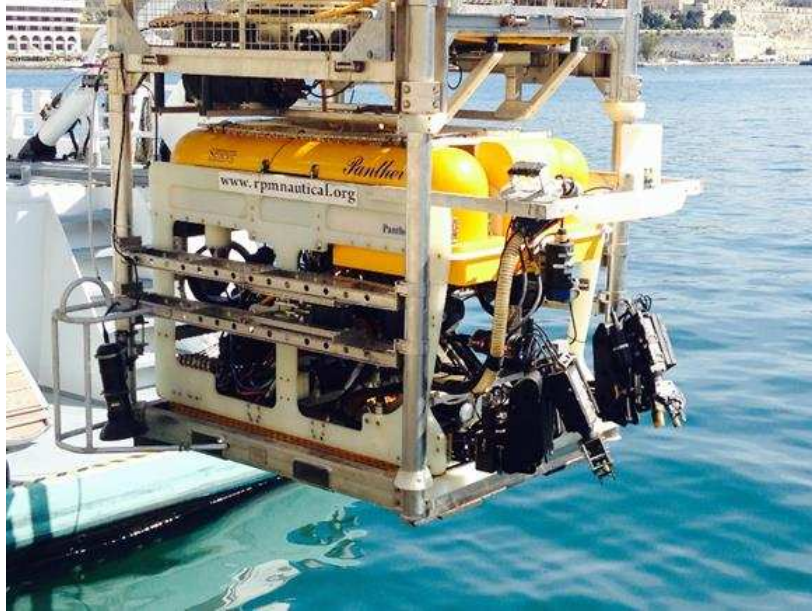
FIGURE 12. ROV being launched from the aft deck of the R/V Hercules (Courtesy of Johnny Dryden and RPM Nautical Foundation, 2014)
