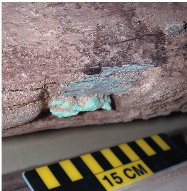
Figure 6. A 5-mm-deep recess protected copper strips at the narrow, pointed end of plank T34 from abrasion. (C. Ward)
