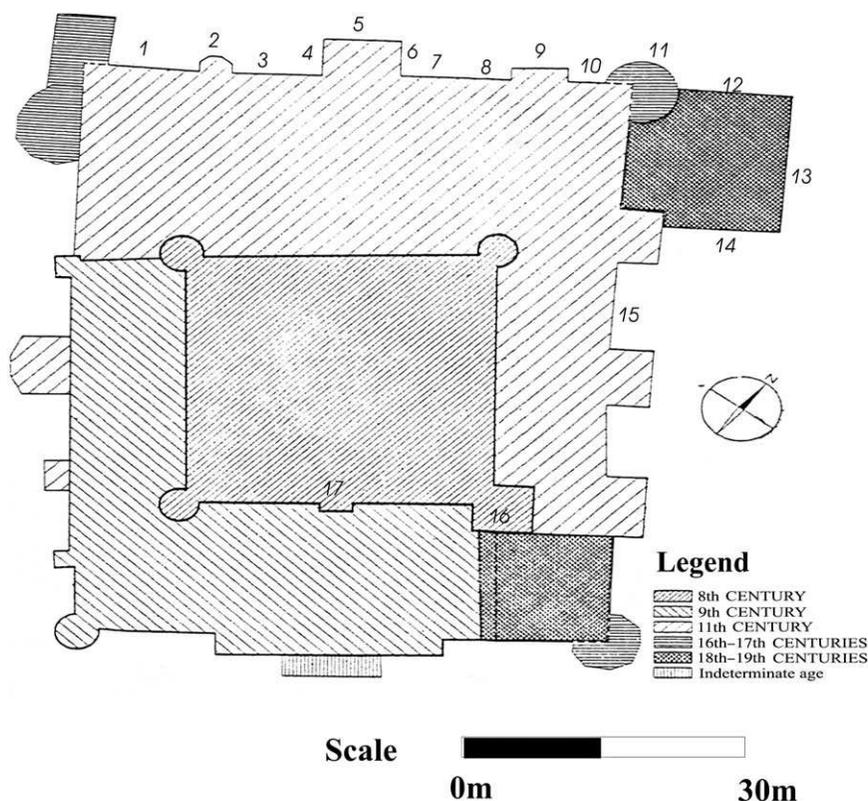
Figure 11 A plan of the Ribat with its different periods of construction and the positions of the blocks measured, from section 1 to section 17 (Lézine 1956).
