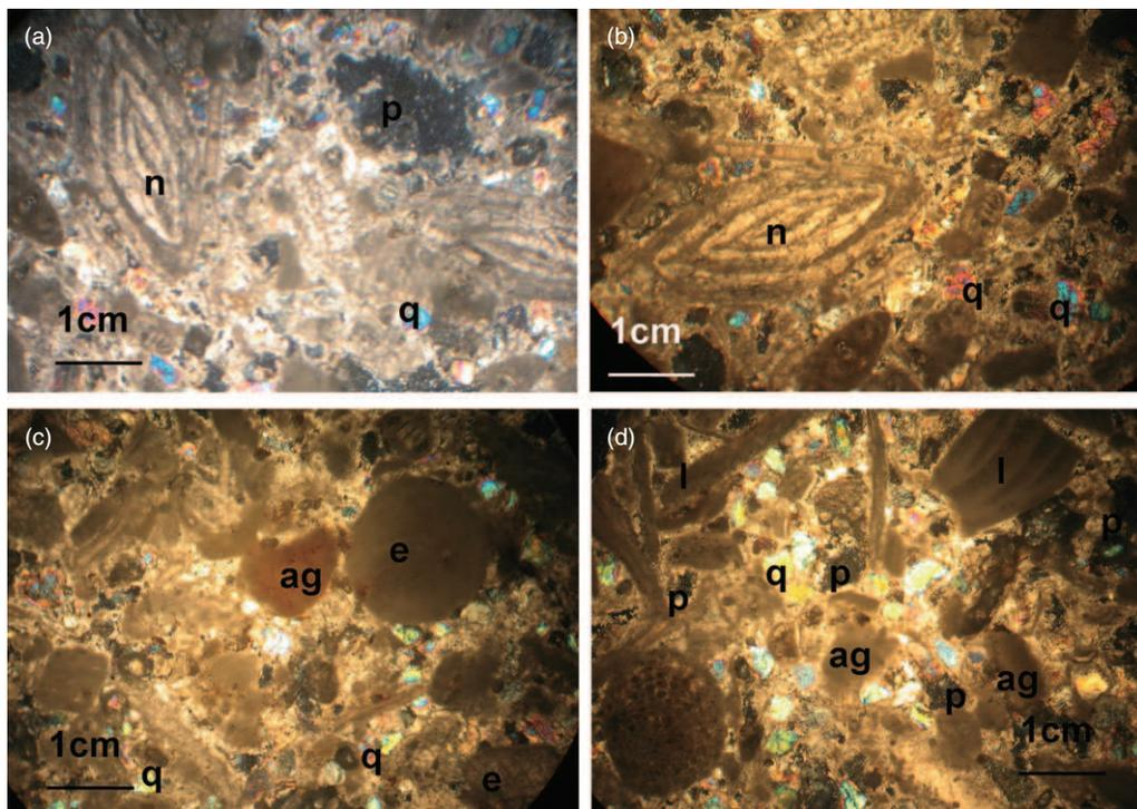
Figure 3 Microfacies of Sidi Ghedamsy stones: limy sandstone (a, b) and sandy limestone (c, d): ag, red algae; e, echinoderm; l, lamellibranch; n, nummulite; p, porosity; q, quartz.
