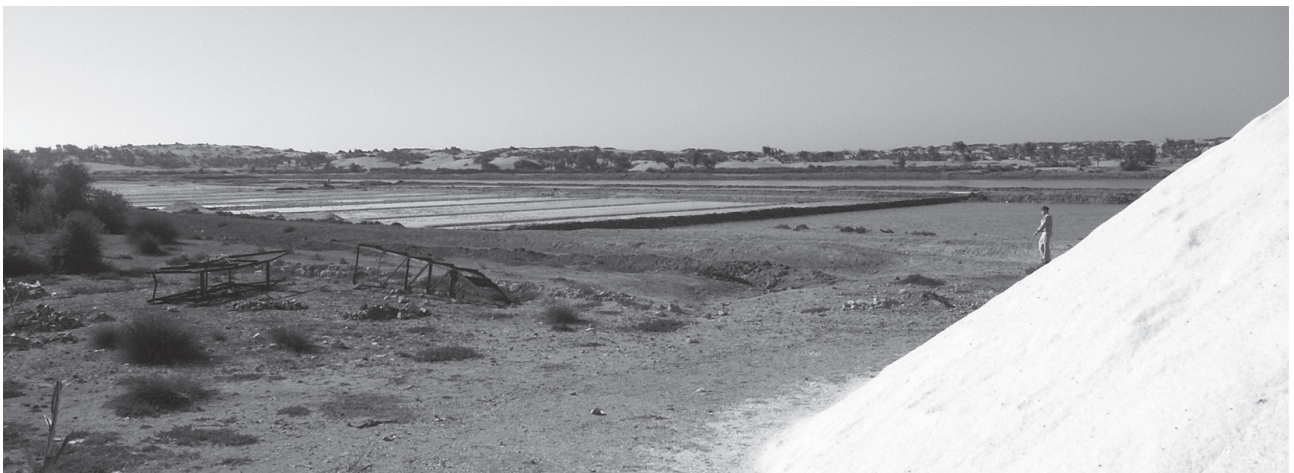
FIG. 119. THE SALINAS AT SIDI ABED, SHOWING, RIGHT TO LEFT, THE PROGRESSIVE STAGES OF THE BRINE CONCENTRATING TO SATURATION (“CORNING” OR CRYSTALLISING), 2007 (PHOTO: AT).
