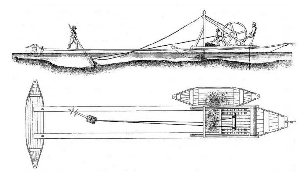
**Figure 3.31:** Eighteenth and nineteenth century dredging equipment used in European fluvial contexts. The vessel immediately adjacent to the 'pull boat' is equipped with a removable bottom, to facilitate the dumping of dredged material at a distal location. Engraving in Billaud and Marguet (2006).
