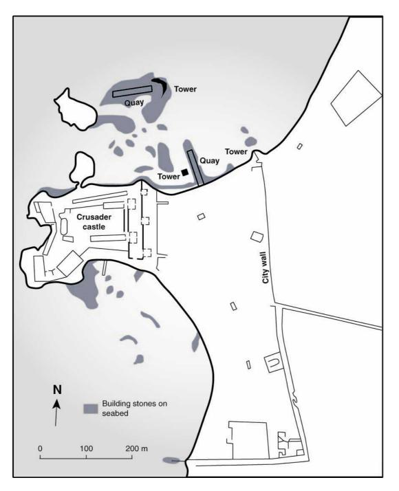
**Figure 3.27:** Athlit's ancient harbour (after Haggai, 2006). Like Tyre, Athlit's harbour lies north of a natural promontory and has yielded some of the best evidence for early Iron Age harbourworks on the Levatine coast. The Phoenician basin is separated into two areas (1) a southern quay and N-S pier; and (2) an eastern quay and northern mole.
