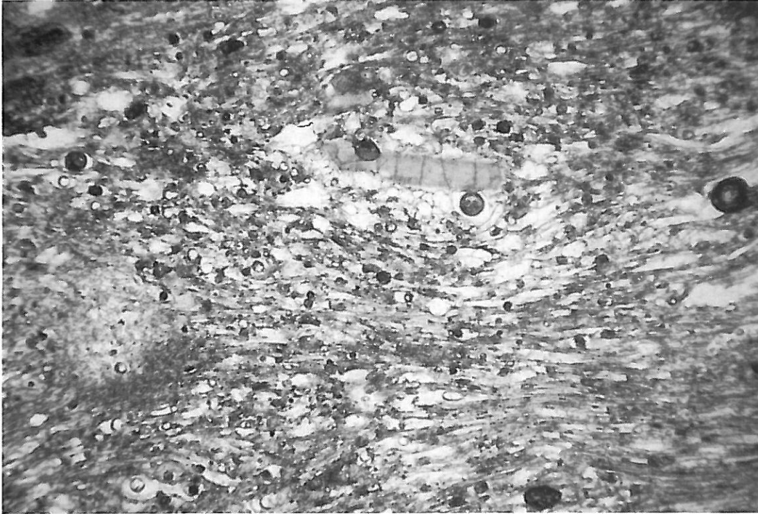
Fig. 6. Crossed polars petrographic slide of a sample of a pozzolana particle from the east face of base level of K5 (M. Grove).
