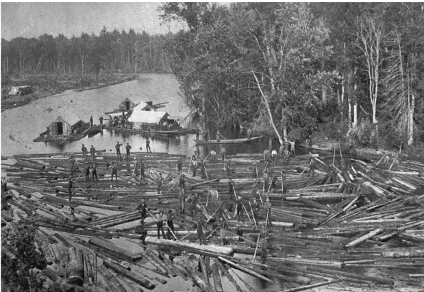
Fig. 13: A typical scenery of a massive river drive. The logs are guided by men with spikes and with small boats. The 1886 drive down the Muskegon River. This site was between Jonesville and Temple. The wanigans were put into the river at Leota, and followed the main drive. Ewart Public Library. Available at http://www.flickr.com/photos/smartee_martee/1867773554/sizes/l/in/photostream/
