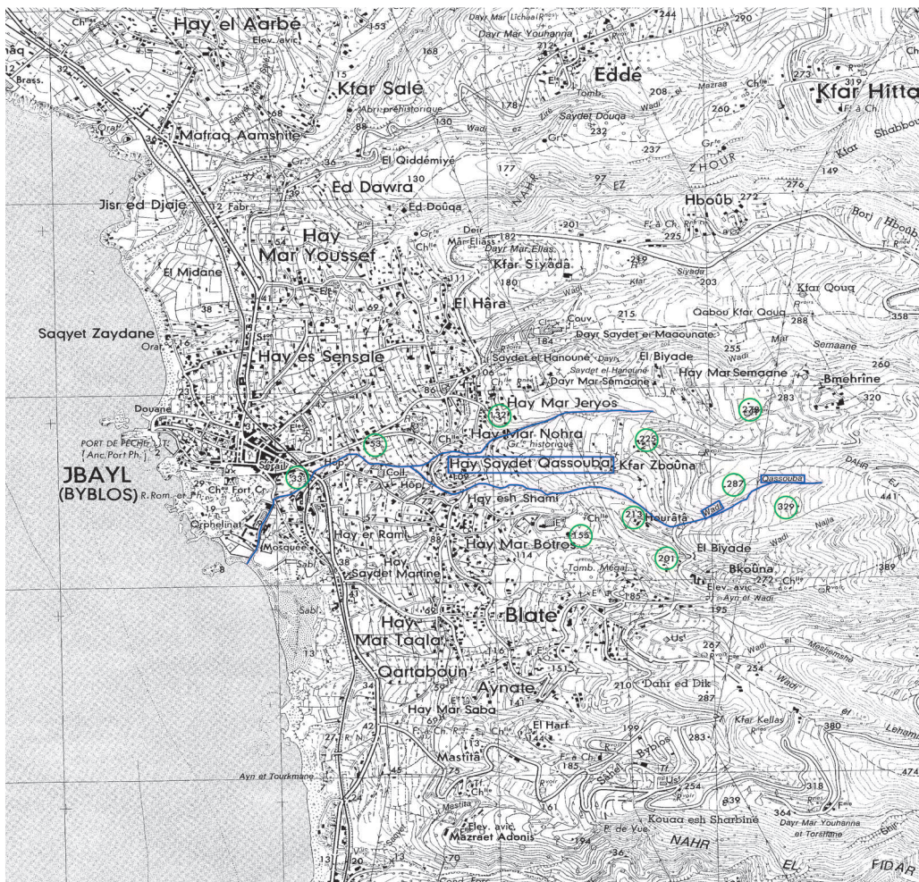
Fig. 16: Map illustrating the Qassouba Wadi topography. The Qassouba valley is drawn in blue. The elevations (circled in green) show the Qassouba starting to flow around 329 m of altitude. The red arrow indicates Nabr el Fidar. Modified from Map of Jbeil 1/20000. Courtesy of Dr. Wissam Khalil
