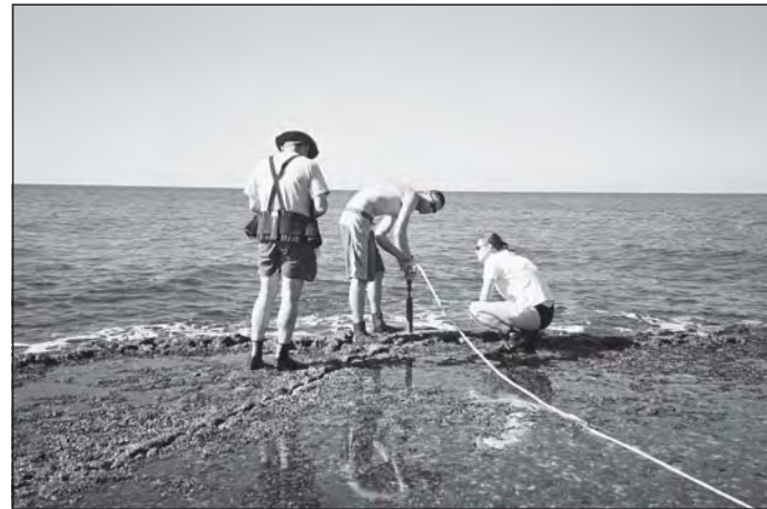
Fig. 2. Drilling cores at the edge of the abrasion platform at Habonim coast (Photo: D. Sivan)
