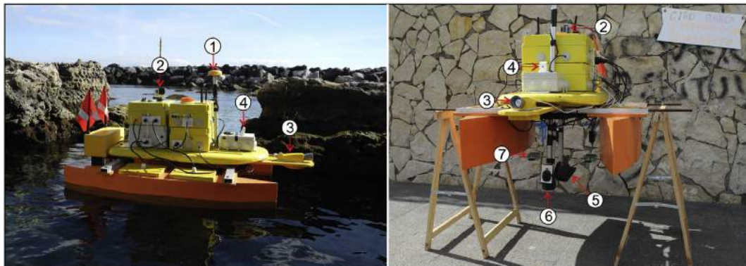
Fig. 3. Marine drone MicroVeGA: 1) GPS receiver; 2)TP-Link 5 GHz; 3) Obstacle detection system Siros 1; 4) emerged camera; 5) Side scan sonar transducer; 6) Single beam echosounder transducer; 7) underwater camera.
