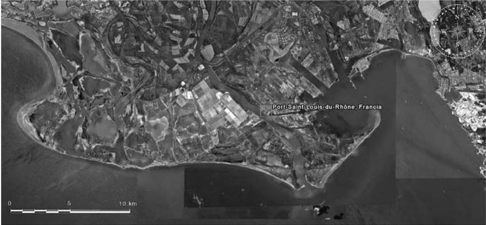
FIG. 3. Example of river delta in tideless seas with lateral spits and bays to be used for port development (the Rhone mouth from Google Earth).
