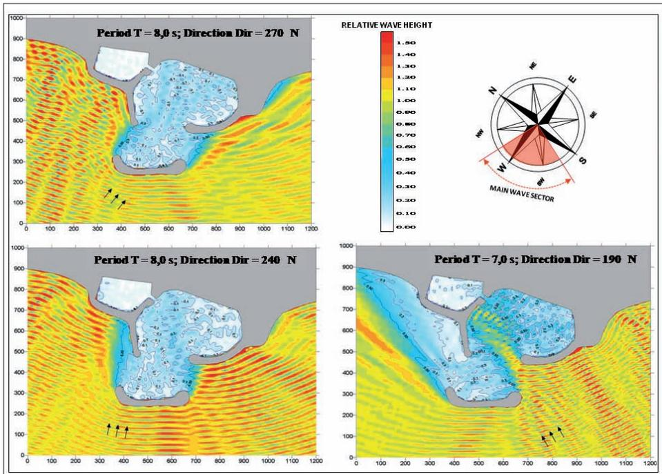
FIG. 11. Wave penetration at *Centumcellae* Port with mathematical model VEGA.
