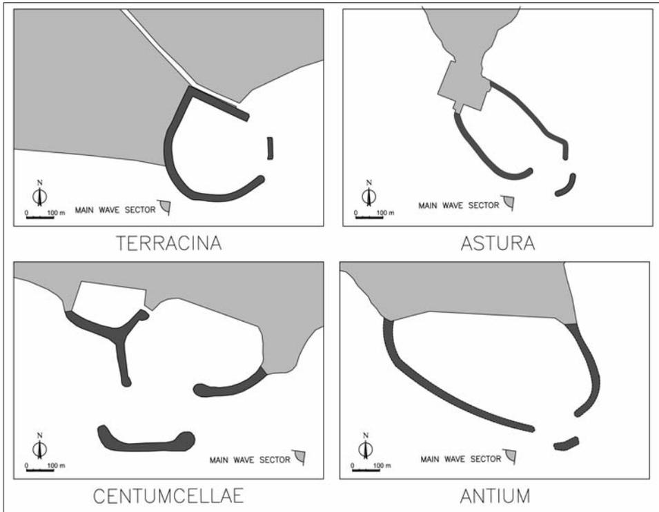
FIG. 8. Roman harbour layouts with double breakwaters and central island.
