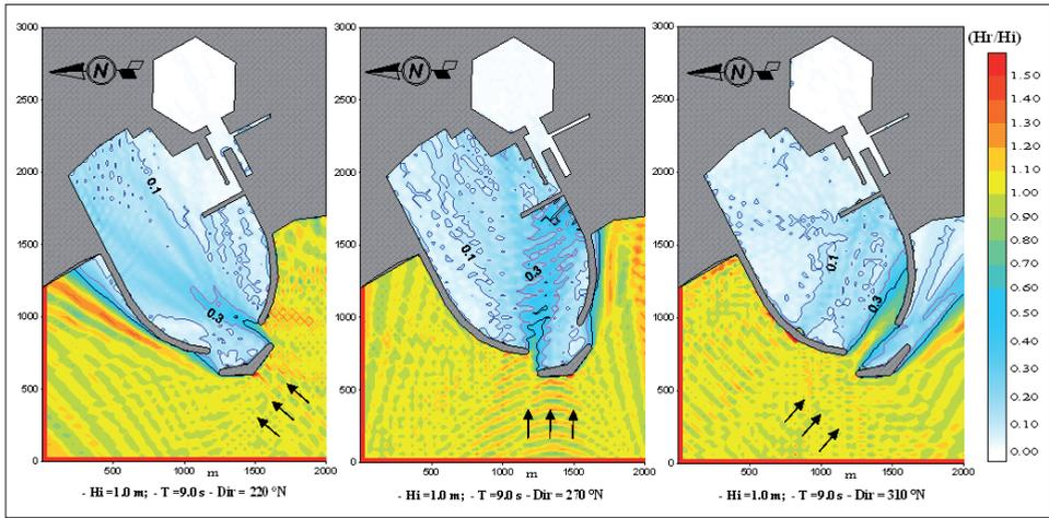
FIG. 10. Wave penetration at *Portus* (according to new proposed port layout) with mathematical model VEGA.
