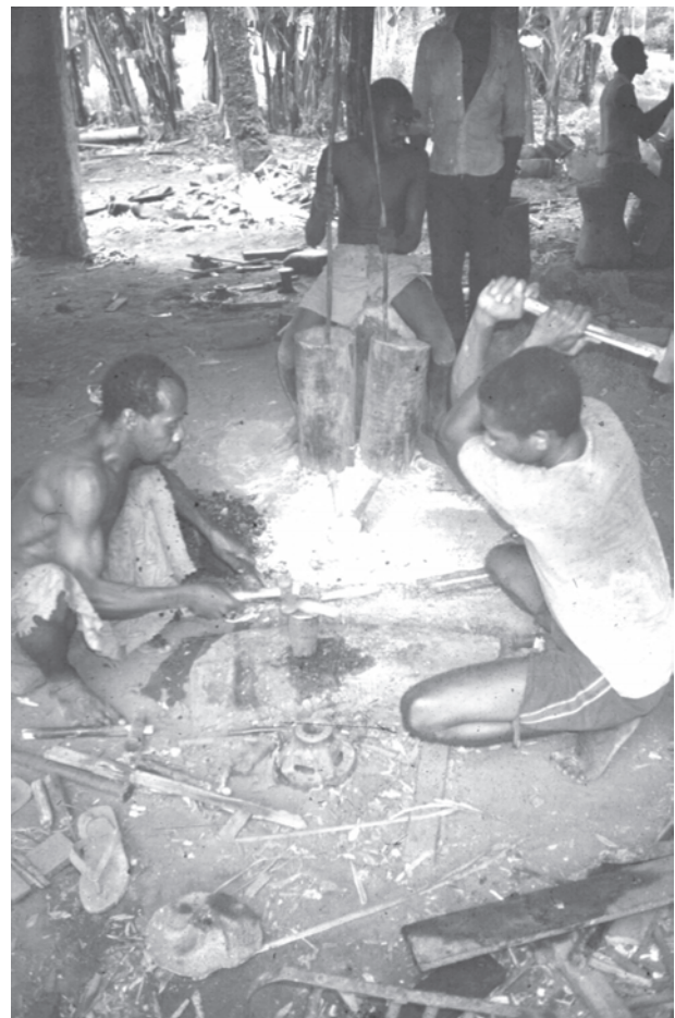
Plate 3.1. Present day iron forging using piston-type bellows, workshop at Kidoti village, north of Unguja Island (Photo 1995).
