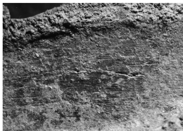
Figure 7. Mechanically cleaned surface of dagger ZP97.232 showing hair-line fracture. Kathy David, ROM.
