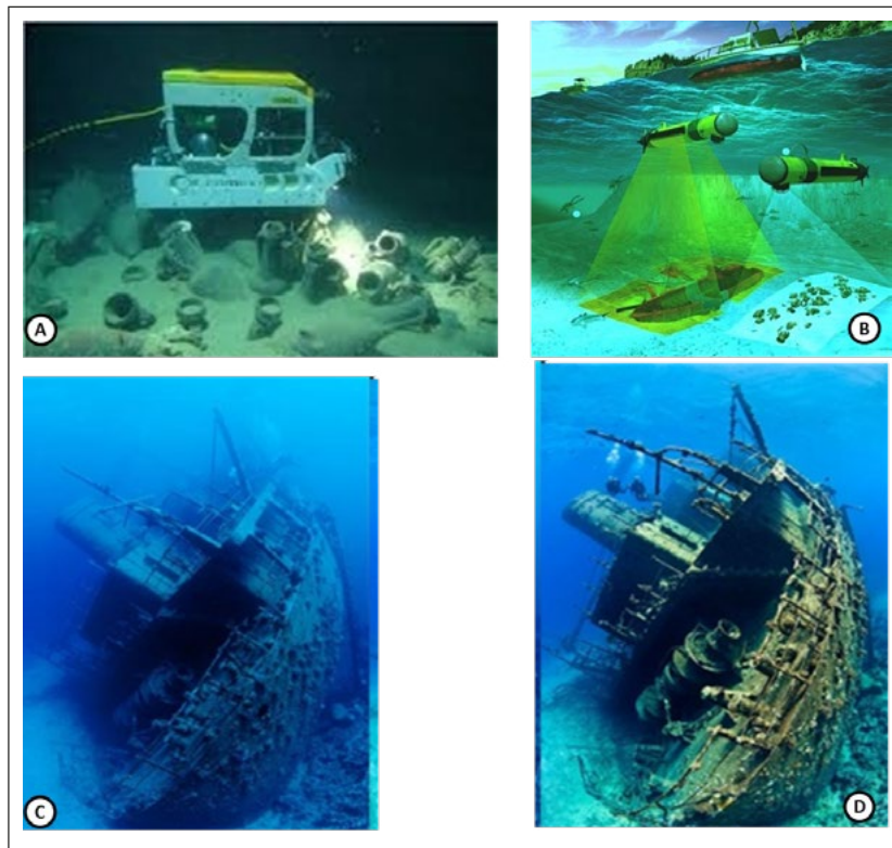
Fig. 7: Examples of under water data acquisition and processing: Remotely operated vehicle based (A) optical under water imaging , (B) SONAR imaging and (C) raw and (D) processed optical images.
