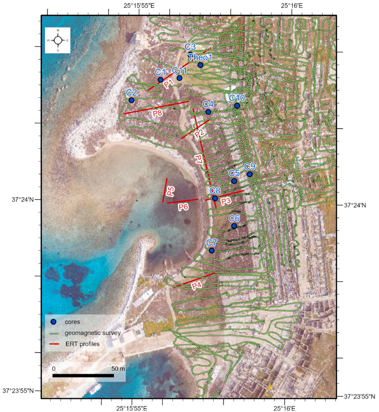
Fig. 3. ERT profiles, electromagnetic survey, and drill core locations. Coordinate system: WGS 1984 UTM Zone 35 N. Basemap: https://sig-delos.efa.gr .
