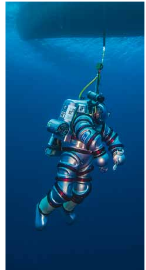
Figs. 1a-b. The Sirius Autonomous Underwater Vehicle produced precision maps of the wreck site and sea floor, while the experimental Exosuit Atmospheric Diving System suggests a possible future direction for archaeology in water to 300 m depth.
