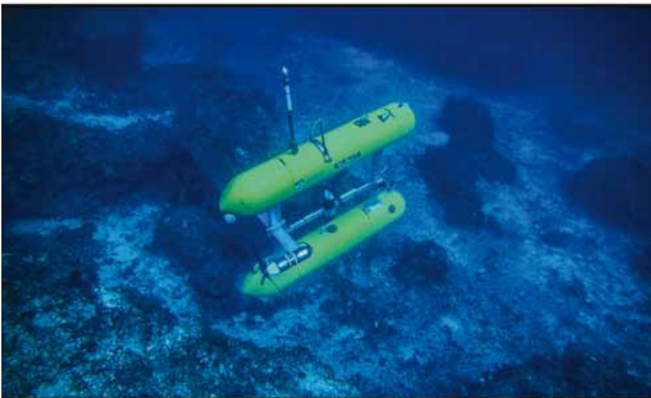
Figs. 1a-b. The Sirius Autonomous Underwater Vehicle produced precision maps of the wreck site and sea floor, while the experimental Exosuit Atmospheric Diving System suggests a possible future direction for archaeology in water to 300 m depth.
