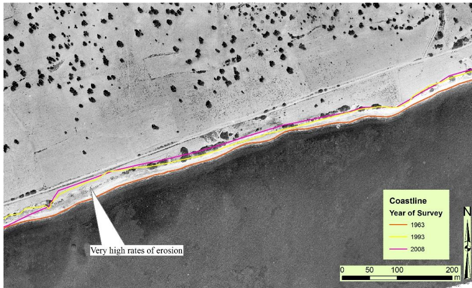
Fig.4.9 High erosion rates between Maroni and Alaminos in the years between 1963 and 2008 (Aerial photographs provided by the DLS – G.M. Andreou).
