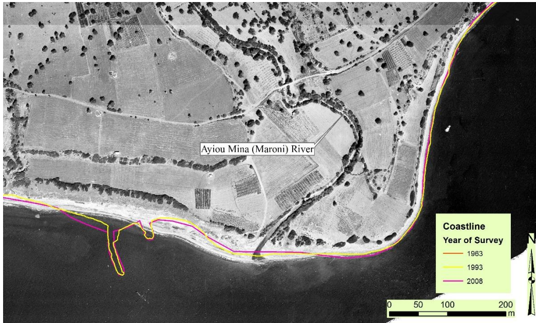
Fig.4.7 Coastal erosion around the mouth of the Maroni River between 1963 and 2008 (Aerial photographs provided by the DLS – G.M. Andreou).
