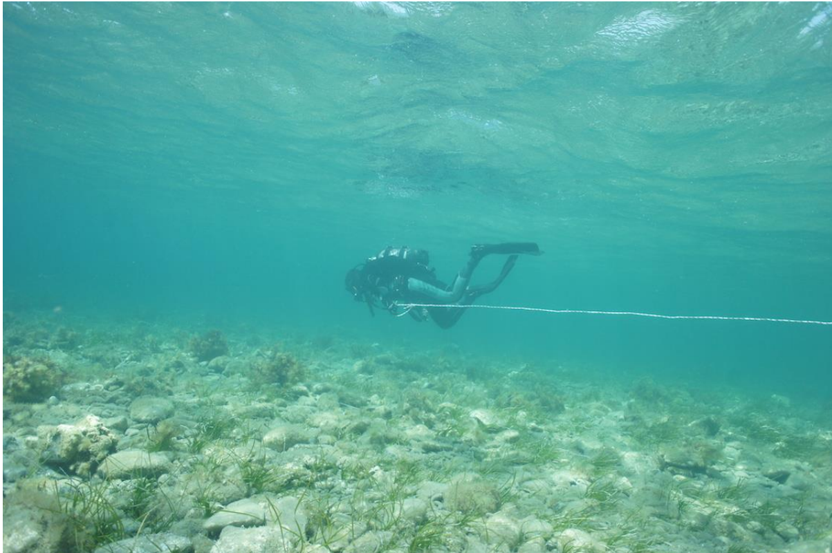
Fig. 3.2. Maria Michael holds one end of a rope 20 metres in length, with three evenly spaced hand-holds. This method of survey assisted the divers in maintaining spacing during transect surveys in lower visibility conditions.
