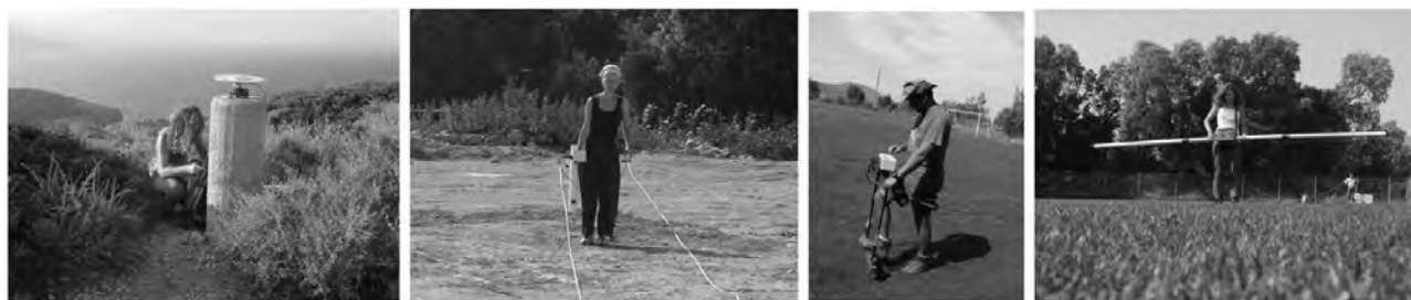
Figure 2. Snapshots from the geophysical survey in the wider area of Istron (from left to right): GPS mapping survey, fluxgate gradiometer survey, electrical resistivity survey and electromagnetic survey.
