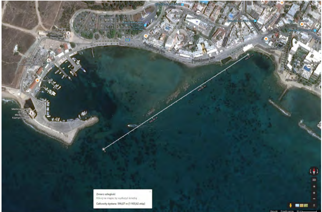
Figure 4: Length of the main ancient breakwater measured on the GoogleEarth satellite image. Created by Ł. Miszk.
