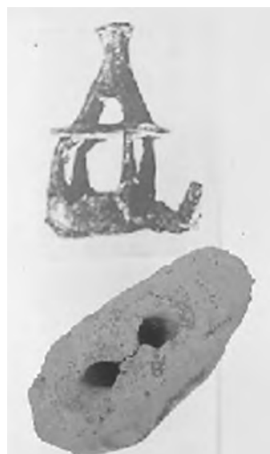
Fig. 46 – The root of the “standing bull” bronzetto and pouring cup and runners from S. Barbara site.
