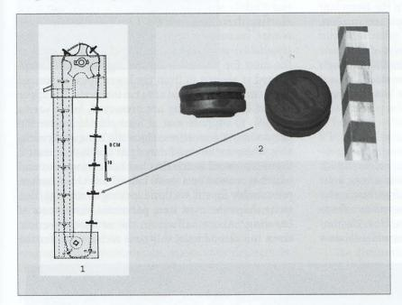
Fig. 2. A wooden disc of a bilge pump, found repaired in the shipyard area.
