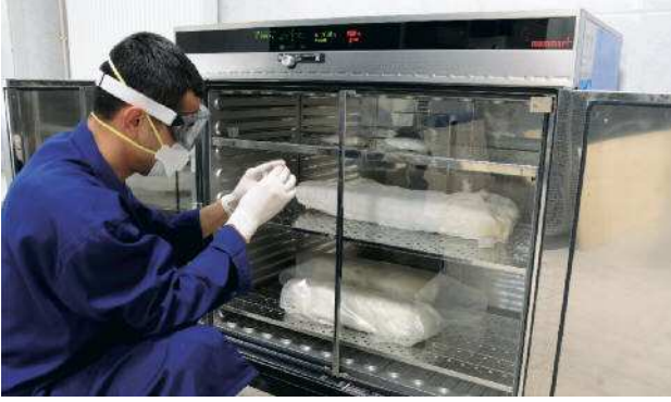
Fig. 16. Woods are being conserved by using Kauramin method.
